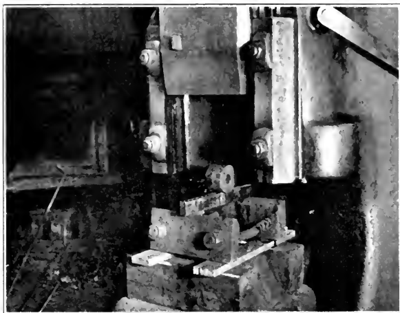
FIGURE 6— Coupon in place for Nick Break Test.
