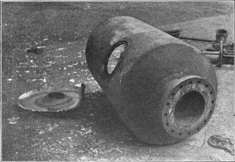
FIG. 4. THE WRECKED SEPARATOR.
