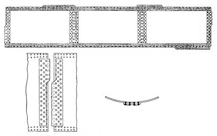
FIG. 4. DETAILS OF COURSE WHICH FAILED.
