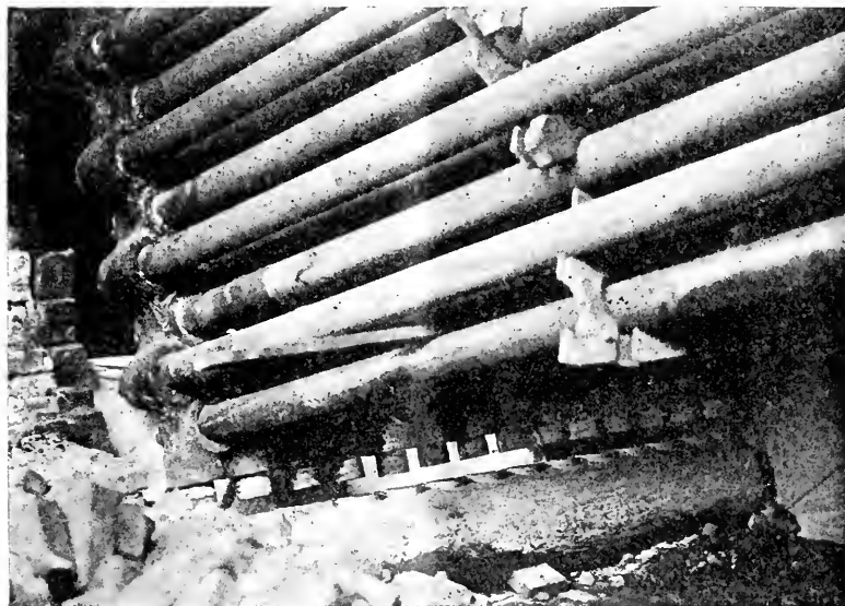
FIG. 1.—ILLUSTRATING THE FAILURE OF NIPPLES.
