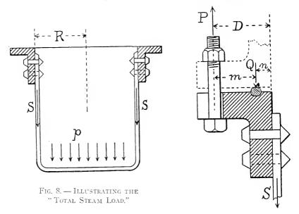
FIG. 9. — THE PRINCIPAL VERTICAL EXTERNAL FORCES.
