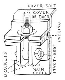
FIG. 1. — Illustrating Certain Details of the Cover-Bolts and Slots.
