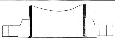
FIG. 10. — ILLUSTRATING A PEENED PIPE.
