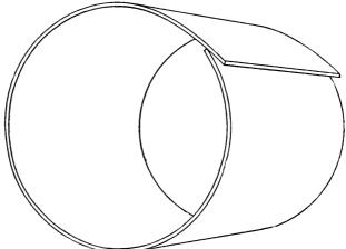
FIG. 4. — Illustrating the "Off-set" of the Lap.
