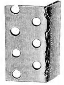
MOST PERFORATED BY A LAP-JOINT CRACK.
