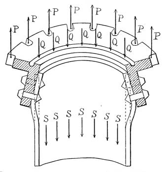
FIG. 10. — THE DISTORTION OF THE RING. (GREATLY EXAGGERATED.)
