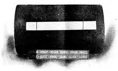
Fig. 8. — Five-inch Pipe; Standard (ok Nearly So) at One End, but Not at the Other.
