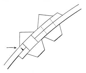
FIG. 11.— ILLUSTRATING THE HIDDEN CRACK WHICH CAUSED THE EXPLOSION. This cut is drawn to scale, one-half the actual size. For a more extended account of lap-joint cracks, see the separate article on this subject, in the present issue.
