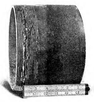
FIG. 9. - EIGHT-INCH PIPE, WHICH COULD BE MADE UP ONLY THREE THREADS.
