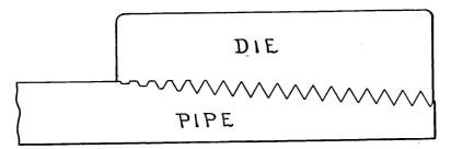
FIG 11. — ILLUSTRATING A COMPLETED PIPE THREAD.
