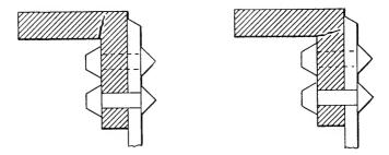
FIGS. 4 AND 5. - METHODS OF FAILURE OF THE RING.
