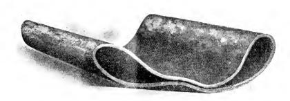
FIG. 1.- SECTION OF A TUBE COLLAPSED BY THE ACTION OF A TUBE CLEANER.
