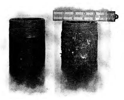
FIG. 6. — THREE-INCH PIPES. (THE ONE ON THE RIGHT COULD BE MADE UP ONLY SIX THREADS. THE OTHER WAS STANDARD, OR NEARLY SO.)
