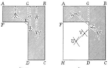
Fig. 20. Fig. 21. Center of Gravity of a Ring-section with Straight Hub.
