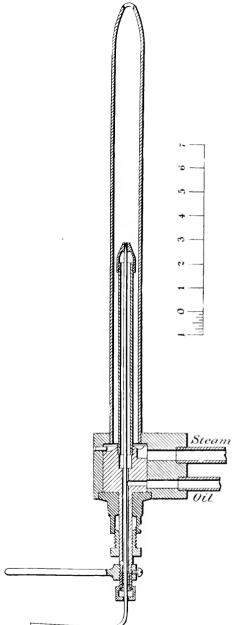
FIG. 4. — THE HAVES BURNER. (Used in Test No. 9.)
