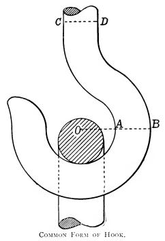
some cases the material was not specially treated. In others it was case-hardened or "carbonized" by heating with granulated raw bone, the small hooks being heated for eight hours and the large one for nine hours. The thickness of the carbonized coating so obtained was about 1/16 of an inch. Some of the hooks were annealed by a separate operation, after the carbonization, and others were
