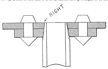
FIG. 2- CORRECT USE OF RE-ENFORCING PIECE.
