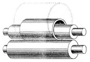
FIG. 4. - ROLLING OUT THE PERFORATED BLANK.
