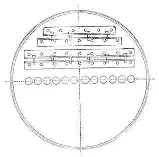
FIG. 2. - SHOWING HORIZONTAL STHFFENING IRONS.
