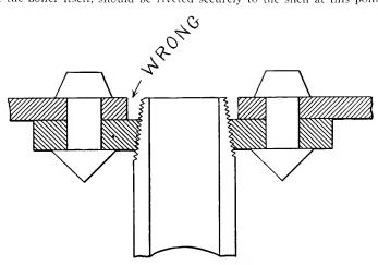
FIG. 1. - WRONG USE OF THE RE-ENFORCING PIECE.
