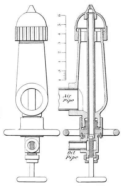
FIGS. 2 AND 3. — THE OIL CITY BOILER WORKS AIR BURNER. (Used in Tests Nos. 1 to 8. inclusive.)
