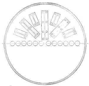
FIG. 1. — SHOWING RADIAL STIFFENING IRONS.
