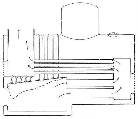
FIG. 2. - SECTIONAL VIEW OF THE "RAMBLER'S" BOILER.
