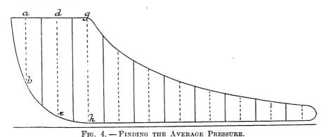
multiplying the average width of the card, in inches, by the number of the spring that was used in taking the card.
