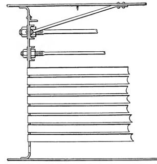
FIG. 2. - SIDE VIEW OF A BOILER HEAD WITH THROUGH BRACES.
