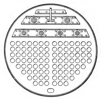
FIG. 1. - A BOILER HEAD WITH THROUGH BRACES.
