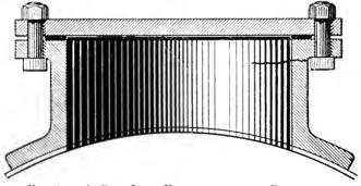
FIG. 1. — A CAST-IRON FLANGE WITHOUT BRACKETS.
