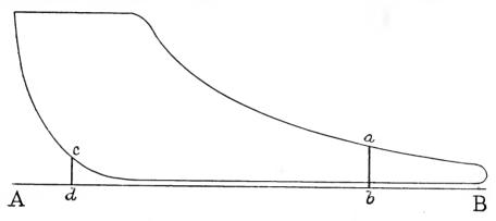
FIG. 1. - TO FIND THE PRESSURE AT ANY POINT IN THE STROKE.
