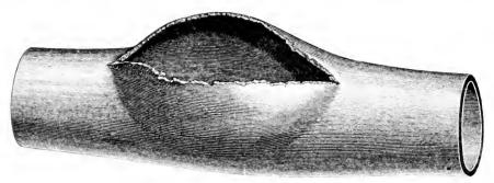
FIG. 6. - A RUPTURED BRASS BLOW-OFF PIPE.
