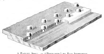
A FAULTY JOINF, AS "PREPARED" TO PASS INSPECTION.
