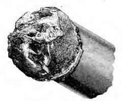
FIG. 1.- A FEED-PIPE NEARLY SEALED UP BY SCALE.
