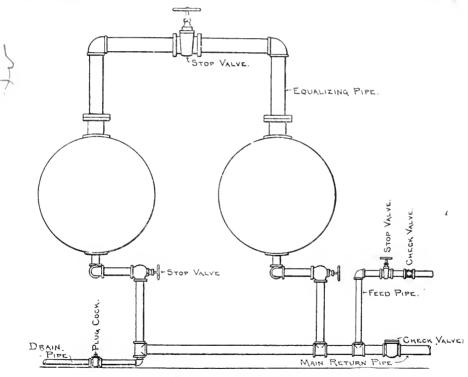
FIG. 1. - ARRANGEMENT OF RETURNS WITH EQUALIZING PIPE.
