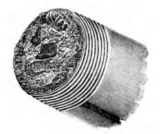
FIG. 3. - A FEED-PIPE CHOKED WITH A STONE-LIKE SCALE.
