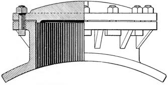
FIG. 2. — A PROPER CONSTRUCTION FOR CAST-IRON MOUTH-PIECES.
