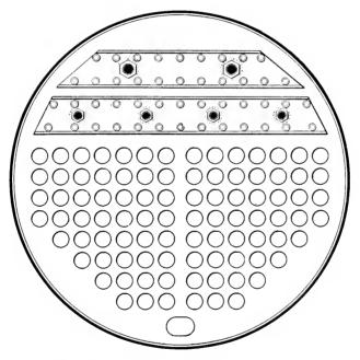
ARRANGEMENT OF THROUGH BRACES AND CHANNEL BARS.
