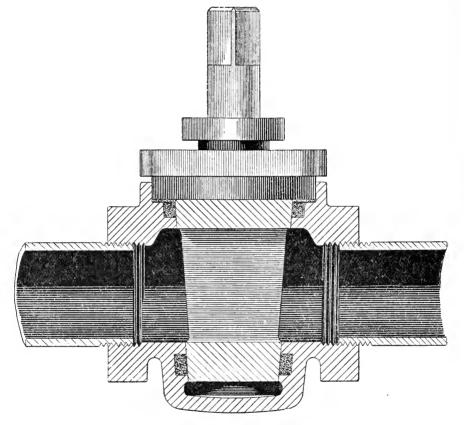
FIG. 2 - A PLUG COCK ON A BLOW-OFF PIPE.
