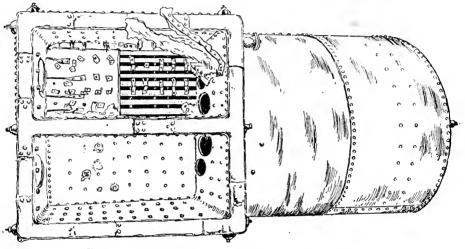
FIG. 3. — THE EXPLODED BOILER, SEEN FROM BELOW.
