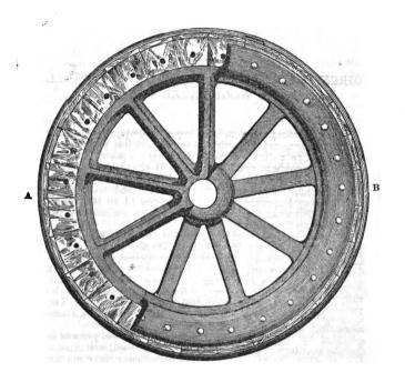
Description—A represents the wheel half in section;  ${\bf B},$  complete; the view being a front elevation.
