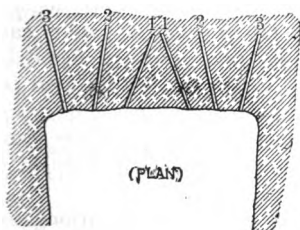
DRILL HOLES IN TUNNEL HEADING
