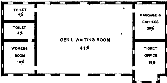
FIG. 160.—DIVISION OF FLOOR AREA RECOMMENDED FOR PASSENGER STATIONS WITH ONE GENERAL WAITING ROOM.
