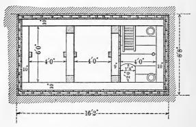
Fig. 91.—Cross-section. Large Main Shaft.
