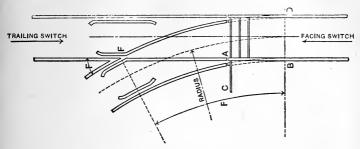
FIG. 131.-STUB SWITCH.
