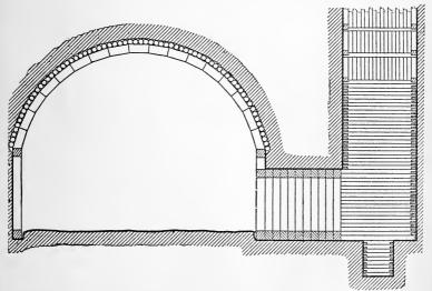
Fig. 90.—Connection with Shaft, Church Hill Tunnel.
