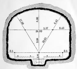
Fig. 87.—Hoosac Tunnel. Section through Solid Rock.
