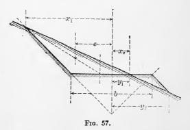
to be irregularly on the outside or on the inside of the curve, and the curvature correction will be correspondingly positive or negative. If the curve is to the right, the correction will be positive or negative according as  $(x_l-x_r)$  is positive or negative; if the curve is to the left, the correction will be positive or nega-
