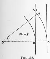
the rails of a frog are free and may be bent to conform to the switch-rail curve, but there is a considerable portion which is fitted to the cast-iron filler, and this portion is always straight. Call the length of this straight portion back from the frog-point f (=FH, Fig. 138). Then we have
