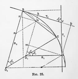
the compound curve having radii of  $R_1$  and  $R_2$  and central angles of  $\mathcal{L}_1$  and  $\mathcal{L}_2$ . Produce the arc AC to n so that  $AO_1n=\mathcal{L}$ . The chord Cn produced must intersect B. The line ns, parallel to  $CO_2$ , will intersect  $BO_2$  so that  $Bs=sn=O_2O_1=R_2-R_1$ . Draw Am perpendicular to  $O_1n$ . It will be parallel to hk.
