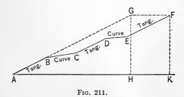
ing the vertical rise from A to G (i.e., HG) in the horizontal distance AH, it requires the horizontal distance AK. addition to the horizontal distance can usually be obtained by proper development, and it should always be done on a ruling grade. Of course it is possible that it will cost more to accomplish this than it is worth, but the engineer should be sure of this before allowing this virtual increase of the grade.
