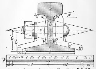
Fig. 119.—Standard Angle-Bar—80-lb. Rail. M. C. R.R.
