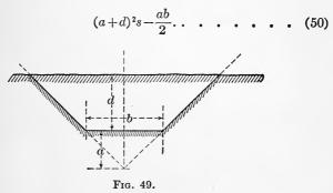
This also follows from Eq. 48 when a=0 and  $\tan \beta = \frac{1}{s}$ . s here represents the "slope ratio," i.e., the ratio of the horizontal projection of the slope to the vertical. A table is very readily formed giving the area in square feet of a section of given depth and for any given width of roadbed and ratio of side-slopes.
