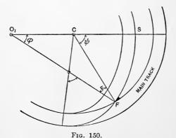
Problem. To find the dimensions of a connecting curve running to the inside of a curved main track; number 9 frog, 4° 30' curve, d = 13',  $g = 4' 8\frac{1}{2}''$ .
