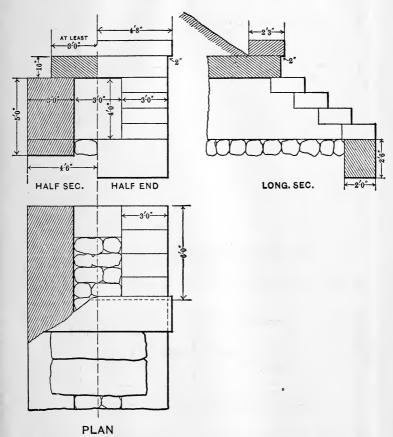
Fig. 100.—Standard Single Stone Culvert (3'×4'). N. & W. R. R. (1890.)
