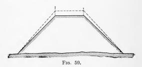
that such figures are only justified because the subsoil settles or because the embankments mush out at the sides, and that if these effects do not occur the levees are permanently higher than designed.
