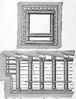
FIG. 93.—TIMBERING FOR TUNNEL HEADING.
