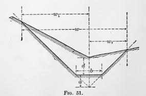
accuracy, is the method of three-level sections. The area of the section is  $\frac{1}{2}(a+d)(w_r+w_l)-\frac{ab}{2}$ , which may be written
