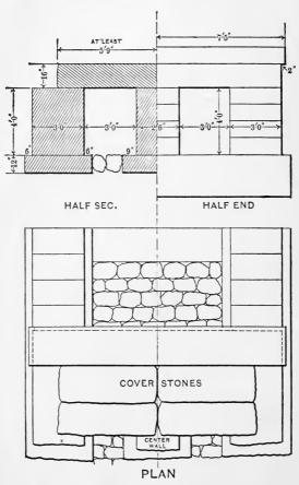
Fig. 100a.—Standard Double Stone Culvert (3' $\times$ 4'). N. & W. R. R. (1890.)
