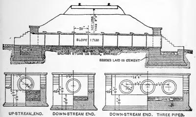
Fig. 98.—Standard Vitrified-pipe Culvert. Plant System. (1891.)
