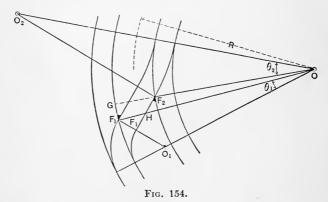
both figures The relative position of the frogs  $F_1$  and  $F_2$  may be determined as follows, the solution being applicable to both Figs. 153 and 154:
