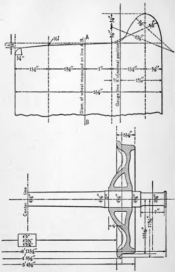
Fig. 204.-M. C. B. Standard Wheel-tread and Axle.
