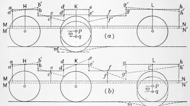
Fig. 195.—Action of Equalizing-Levers.
