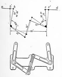
Fig. 171.—STANDARD PIPE COMPENSATOR.
