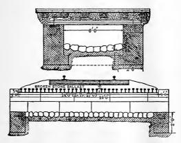
Fig. 101.—Standard Old-rail Culvert. N. & W. R.R. (1895.)
