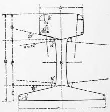
Fig. 113.—Am. Soc. C. E. Standard Rail Section.
