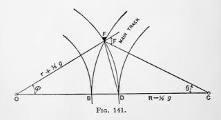
track. In this demonstration the switch-rails will be considered as uniformly circular from the switch-points to the frog-point.
