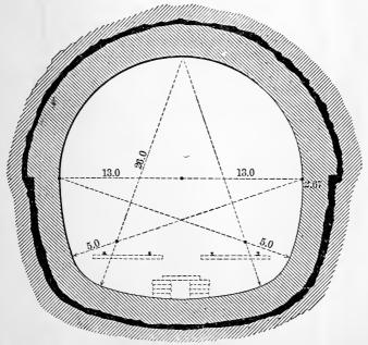
Fig. 88.—Hoosac Tunnel. Section through Soft Ground.
