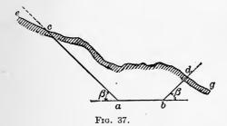
how irregular; ab represents the position and width of the required roadbed; ac and bd represent the "side slopes" which begin at a and b and which intersect the natural surface at such
