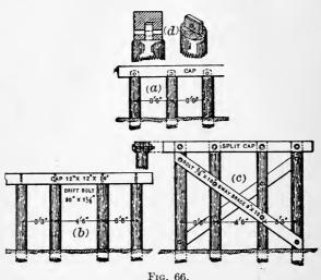
of 8 or 10 feet four piles may be used without sway-bracing, as in Fig 66 (b), if the piles have a good bearing. For heights greater than 10 feet sway-bracing is generally necessary. outside piles are frequently driven with a batter varying from 1:12 to 1:4.
