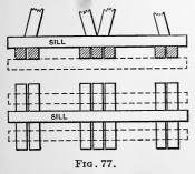
built by the Louisville and Nashville R. R. Eight blocks 12"×12"×6' are used under each bent. When the ground is very soft, two additional timbers (12"×12"×length of bent-sill), as shown by the dotted lines, are placed underneath. The number required evidently depends on the nature of the ground.
