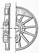
Fig. 199.—Section of Locomotive-driver.
