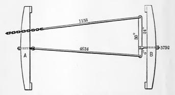
Fig. 205.—Sketch of Mechanism of Hand-brake.
