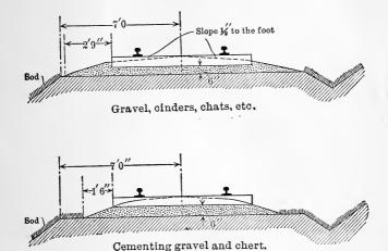
Fig. 108.—Cross-sections of Ballast for Class "C" Roads.
