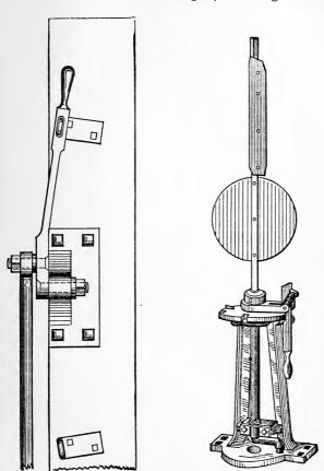
Fig. 134.—Ground Lever for Throwing A Switch.
