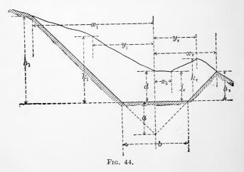
bed and side slopes gives three straight lines. The intersection with the natural surface is in general an irregular line. On smooth regular ground or when approximate results are acceptable this line is assumed to be straight. According to the irreg-
