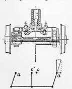
Fig. 183.—Action of Shifting Center.
