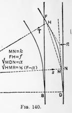
must be placed during the brief period between the running times of trains, it will be easier to joint up to the frog a piece of rail at one or both ends of just such a length that they may be quickly substituted for an equal length of rail taken out of When the frog is thus in place the point Hbecomes located. The chord MH may be measured on the ground. The curve between M and H is of known radius.
