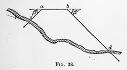
points (c and d) as will be determined by the required slope angle  $(\beta)$ .
