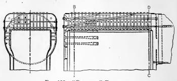
$\begin{array}{ccc} & \text{Fig. 192.--}\text{``Belpaire'' Fire-box.} \\ \text{Half-section through } AB. & \text{Half-section through } CD. \end{array}$
