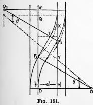
Fig. 151.) The turnouts are as usual. The cross-over track may be straight, as shown by the full lines, or it may be a reversed curve, as shown by the dotted lines. The reversed curve shortens the total length of track required, but is somewhat objectionable. The first method requires that both frogs must be equal. The second method permits unequal frogs, although equal frogs
