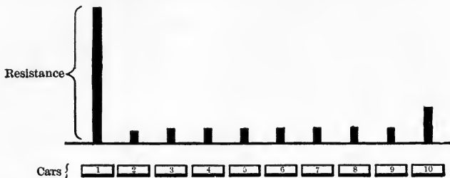
FIG. 224.—Relative Resistance Offered by the Several Cars of a Train.
