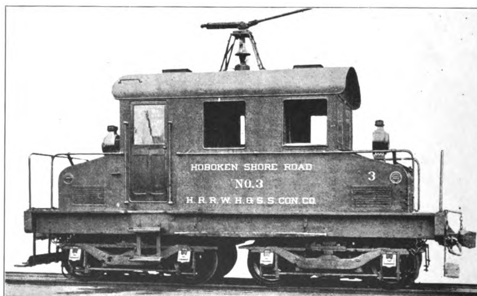
Fig. 4671. Baldwin-Westinghouse Electric Locomotive for the Hoboken Shore Road. Weight, 120,000 lbs.; Diameter of Drivers, 36 in.; Wheel Base, 19 ft.; Drawbar Pull, Starting, 24,000 lbs.; Drawbar Pull, Running, 14,500 lbs.; No. of Motors 4.
