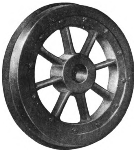
Fig. 4568. Steel Tired Wheel with Wrought Iron or Cast Steel Spoke Center. Double Lip Retaining Ring.
