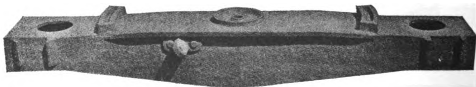
Fig. 4421. Cast-Steel Truck Bolster, Box Section. American Steel Foundries.
