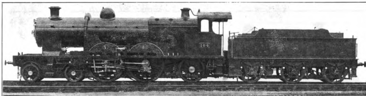
Fig. 5054. Ten-Wheel, Four-Coupled, De Glehn, Four-Cylinder Balanced Compound Locomotive. Great Western Railway. Cylinders 14 13-16 in. and 23 \frac{3}{8} in. x 25 3-16 in.; Working Steam Pressure 227 lbs. per sq. in.; Total Heating Surface 2,755.7 sq. ft.; Weight on Drivers 75,040 lbs.; Total Weight 159,940 lbs.
