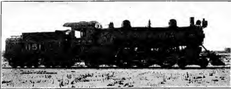
Modern 4-6-2 Passenger Engine, on Canadian Pacific Railway. Cylinders, 21 x 28 Inches; Drivers, 69 inches; Weight of Engine, 214,300 Pounds Steam Superheated
