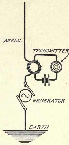
Fig. 7. Transmitter Inductively Associated with Aerial
