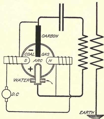
Fig. 36. Poulsen Direct-Current Method of Generating Oscillations
