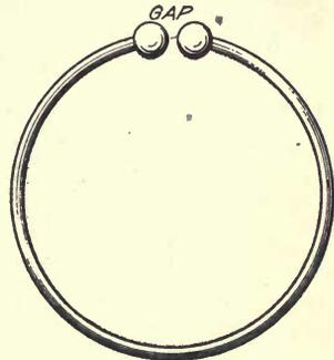
Fig. 6. Hertz Resonator
