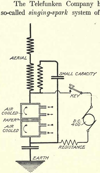
Fig. 61. Von Lepel Oscillation Generator Circuit
