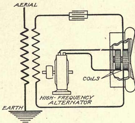
Fig. 13. Heterodyne Receiver Circuit
