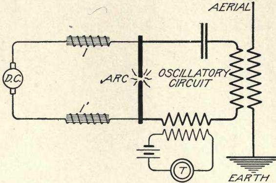
Fig. 9. Transmitter Inductively Associated with the Closed Oscillatory Circuit
