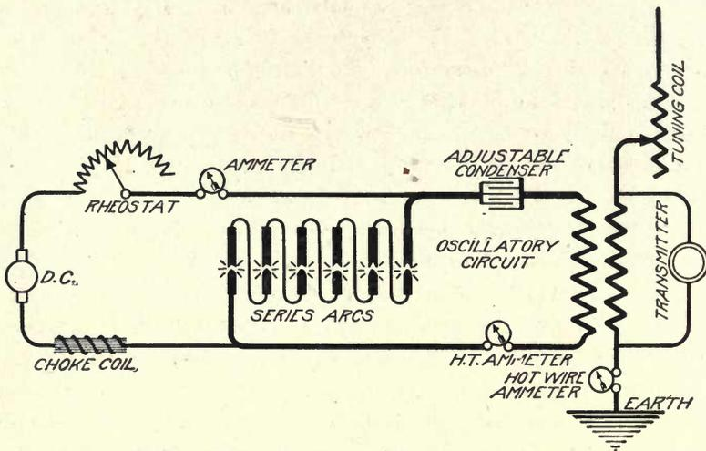
Fig. 14. Transmitter Circuit of the Telefunken System
