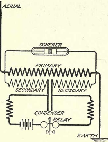
Fig. 19. Marconi Receiver-Circuit with Jigger
