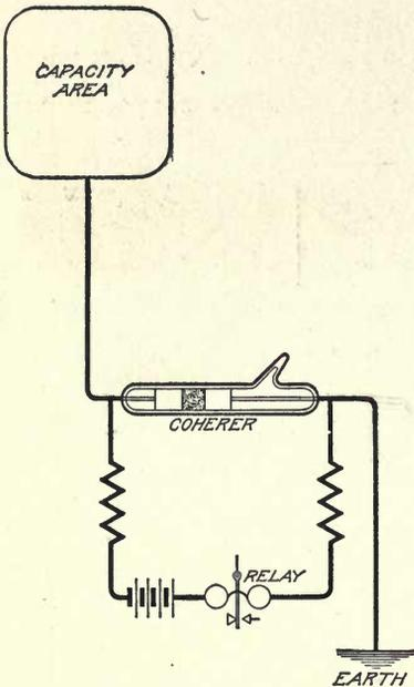
Fig. 16. Earthed Receiving Circuit
