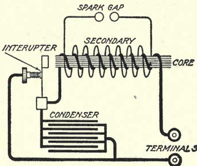
Fig. 23. Diagram of Induction Coil Showing Condenser Circuit
