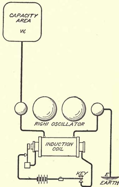
Fig. 15. Diagram Showing the Earthed Oscillator
