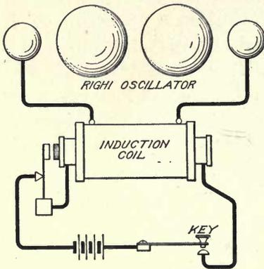
Fig. 12. Early Marconi Transmitter Circuit
