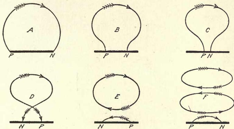
Fig. 5. Formation of Closed Loops of Electric Strain
