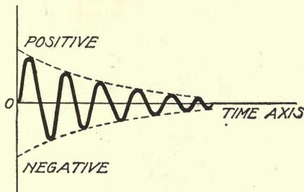
Fig. 3. Curve Representing an Oscillatory Discharge
