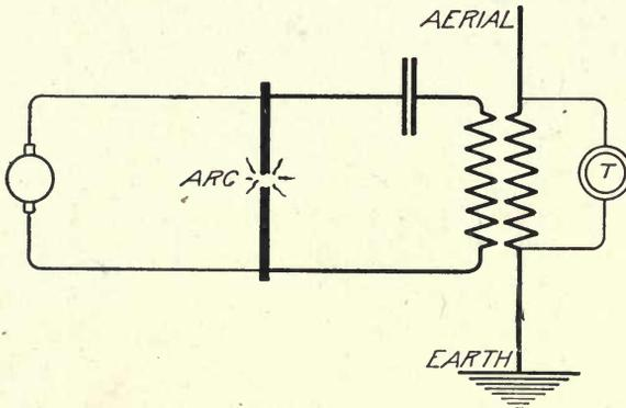
Fig. 10. Transmitter Shunted across the Aerial Inductance
