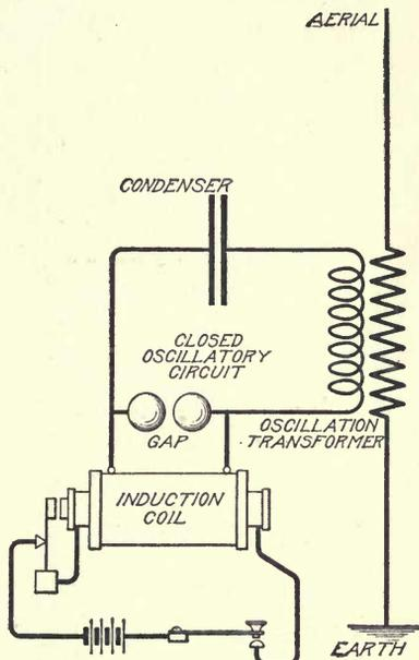
Fig 20 Marconi-Braun Inductive Transmitting Antennae
