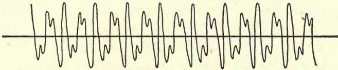
Fig. 5. Oscillogram of a Telephone Current
