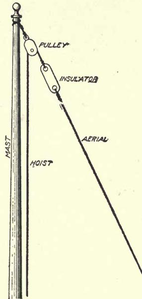
Fig. 41. Single Wire Experimental Aerial
