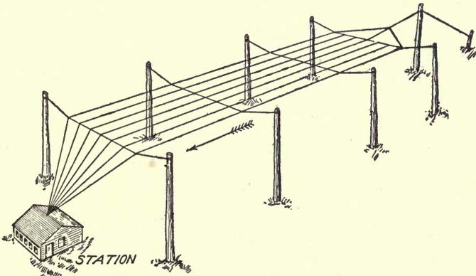
Fig. 42. Antennae Construction for High-Power Station
