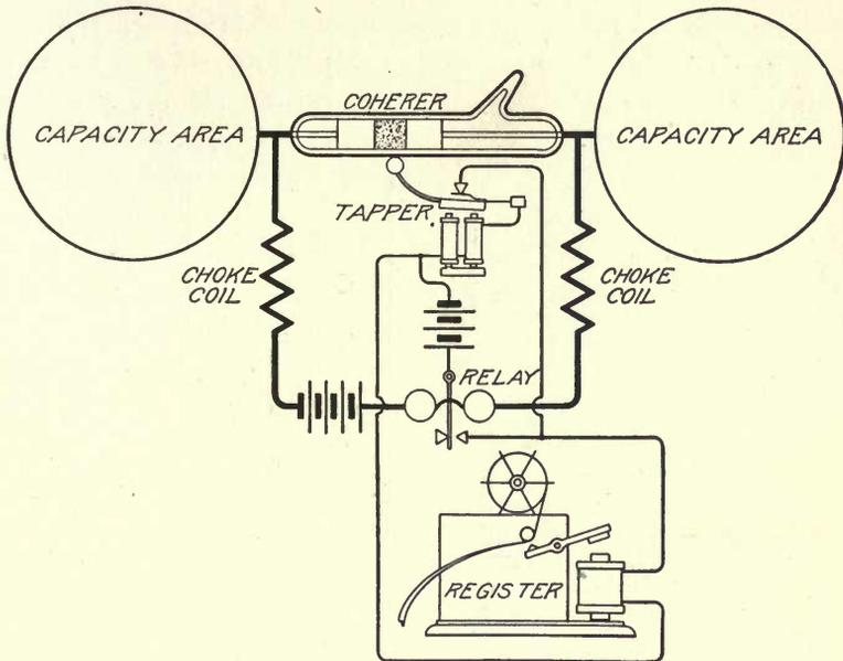
Fig. 13. Early Marconi Receiving Circuit
