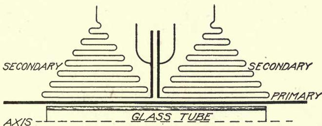
Fig. 18. Diagram of Oscillation Transformer Winding
