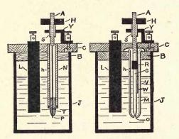
Fig. 41. Construction of Electrolytic Interrupters.
