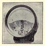
Fig. 87. United Wireless Hot Wire Ammeter.
