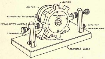
Fig. 159. Details of Rotary Gap.
