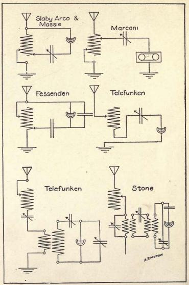
Plate IV. Receiving Circuits. (Straightaway Aerial.)
