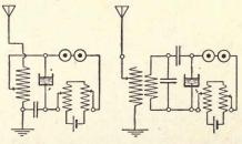
Fig. 93. Electrolytic Detector Circuits.
