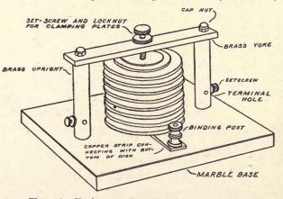
Fig. 156. Explanatory Drawing of Quenched Gap.
