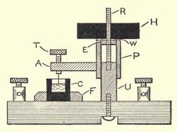
Fig. 100. Electrolytic Detector.
