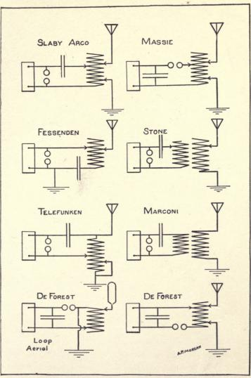
Plate III. Transmitting Circuits.
