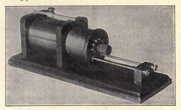
Fig. 134. A Highly Efficient Form of Loose Coupler,
