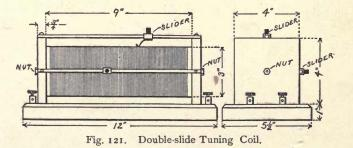
and cause it to better retain its shape. The tube is held tightly between the two heads by means of a brass rod which passes through the center and is clamped by two nuts.
