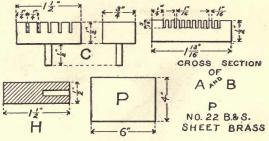
Fig. 140. Details of Variable Condenser.
