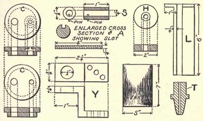
Fig. 42. Details of Electrolytic Interrupters.
