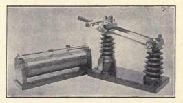
Fig. 77. Shoemaker Tuning Coil and Aerial Switch.
