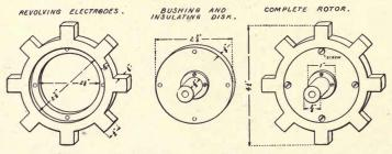
Fig. 158. Details of Revolving Parts of Rotary Gap.
