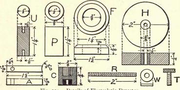
Fig. 101. Details of Electrolytic Detector.
