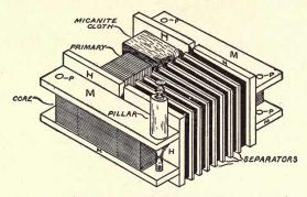
Fig. 49. Transformer with One Secondary removed.
