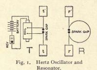
take. T represents the transmitting apparatus and R the receptor. At the transmitting station a telegraph key is placed in series with a battery and an induction coil. Two large metal plates, t and t', are connected to the oppo-
