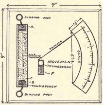
Fig. 81. Meter with Case Removed.
