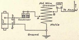
Fig. 63. Closely Coupled Tuning Circuit.
