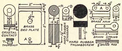
Fig. 89. Details of Universal Detector.
