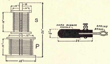
Fig. 64. Loosely Coupled Transmitting Helix and Contact Clip.
