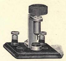
Fig. 94. Electrolytic Detector.
