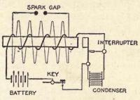
Fig. 25. Diagram of an Induction Coil.
