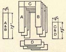
Fig. 44. Assembly and Dimensions of Core.
