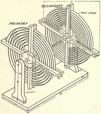
Fig. 152. Details of Oscillation Helix Construction.
