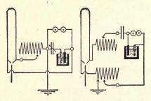
Fig. 97. Shoemaker Detector Circuits.
