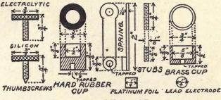
Fig. 90. Parts of Universal Detector.
