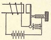
Fig. 33. Simple Interrupter.
