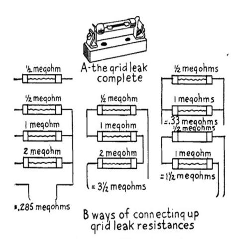
Fig. 42.—Grid Leaks and How to Connect Them up.
