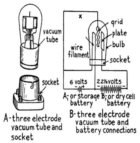
Fig. 38.—Three Electrode Vacuum Tube Detector and Battery Connections.
