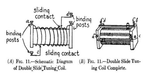
When connecting in the tuning coil, only the post *a* or the post *b* is used as may be most convenient, but the other end of the wire which is connected to a post is left free; just bear this point in mind when you come to connect the tuning coil up with the other parts of your receiving set. The tuning coil is shown complete at *B* and it costs \$3.00 or \$4.00. A *triple slide* tuning coil constructed like the double slide tuner just described, only with more turns of wire on it, makes it
