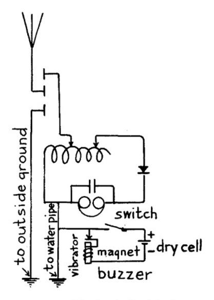
Fig. 17.--Adjusting the Receiving Set.
