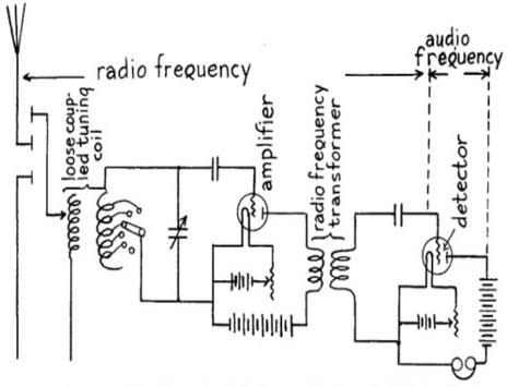
(A) Fig. 45.—Wiring Diagram for a Radio Frequency Transformer Amplifying Receiving Set.
