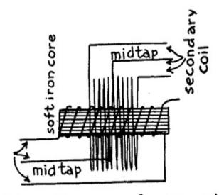
A. wiring diagram of microphone transformer
