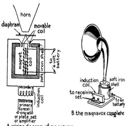
A. wiring diagram of magnavox
