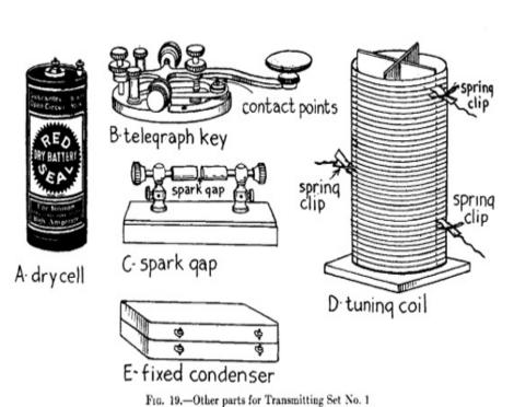
The Telegraph Key.--You can use an ordinary Morse telegraph key for the sending set and you can get one with a japanned iron base for \$1.50 (or better, one made of brass and which has 1/8-inch silver contact points for \$3.00. A key
