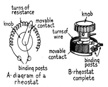
Fig. 40.—Rheostat for the A or Storage Battery Current.
