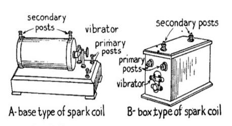
(A) and (B) Fig. 18.—Types of Spark Coils for Set. No. 1.
