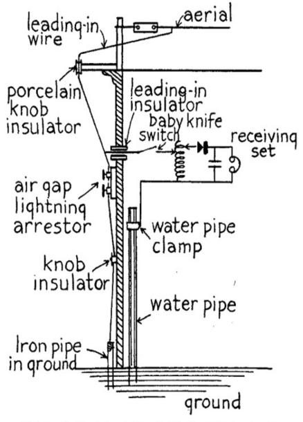
(B) Fig. 6.-Receiving Aerial with Air Gap Lightning Arrester.
