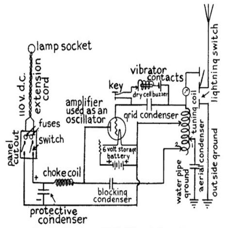
Fig. 76.—Experimental C. W. Telegraph Transmitter.
