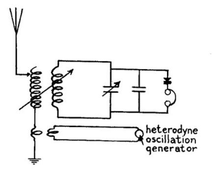
Fig. 74.—Separate Heterodyne Oscillator.
