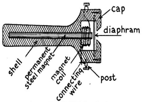
Fig. 62.—Cross-section of Bell Telephone Receiver.
