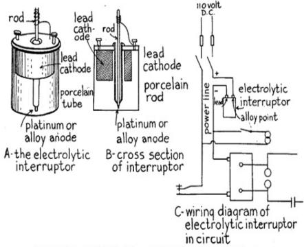
Fig. 23.-Using 110 Volt Direct Current with an Alternating Current Transformer.
