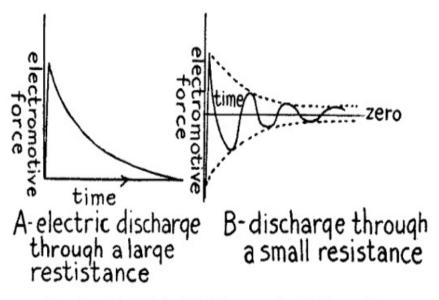
Fig. 33.—The Effect of Resistance on the Discharge of an Electric Current.
