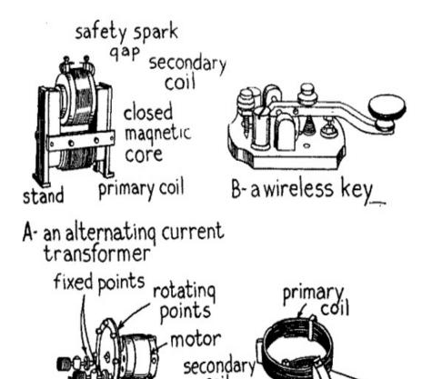
Fig. 21.—Parts for Transmitting Set No. 2.
