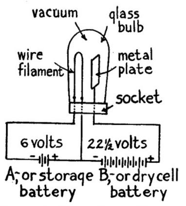
Fig. 37.—Two Electrode Vacuum Tube Detectors.
