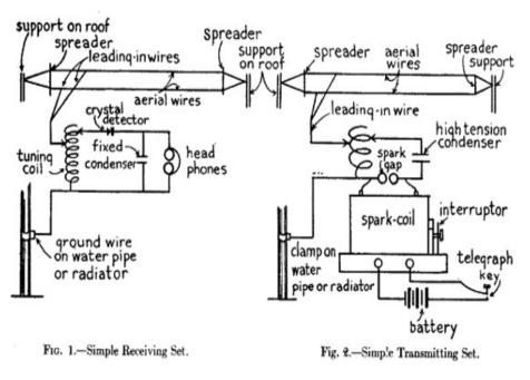
A tuning coil of the simplest kind consists of a single layer of copper wire wound on a cylinder with an adjustable, or sliding, contact, but for sharp tuning you need a *loose* coupled tuning coil. Where a single coil tuner is used a fixed condenser should be connected around the telephone receivers. Where a loose coupled tuner is employed you should have a variable condenser connected across the closed oscillation circuit and a fixed condenser across the telephone receivers.
