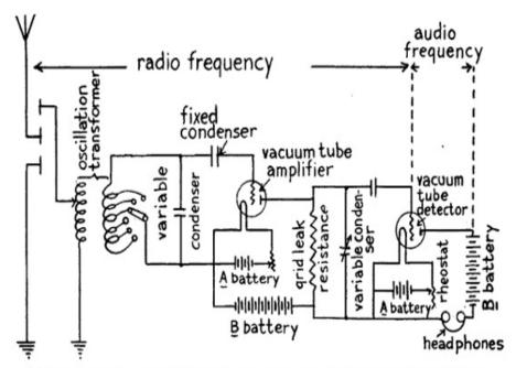
(A) Fig. 44.—Vacuum Tube Detector Receiving Set with One Step Amplifier (Resistance Coupled).
