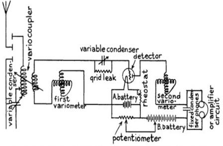
Fig. 56.—Short Wave Regenerative Receiving Set (two Variometer and two Variable Condensers.)
