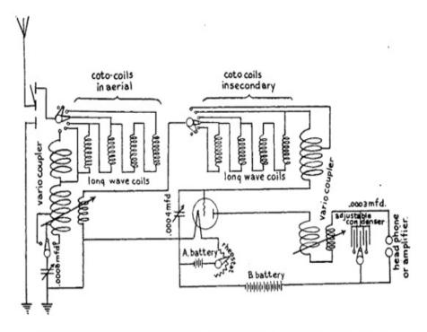
Fig. 59,—Wiring Diagram Showing Long Wave Receptor with Variocouplers and 8 Bank-wound Inductance\_Coils
