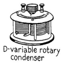
(C) and (D) Fig. 13.—The Variable Rotary Condenser.
