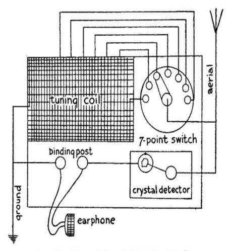
Fig. 99.—Schematic Layout of \$5.00 Receiving Set.
