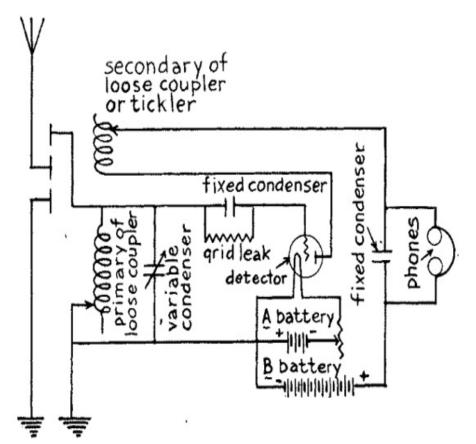
Fig. 48.—Simple Regenerative Receiving Set. (With Loose Coupler Tuner.)
