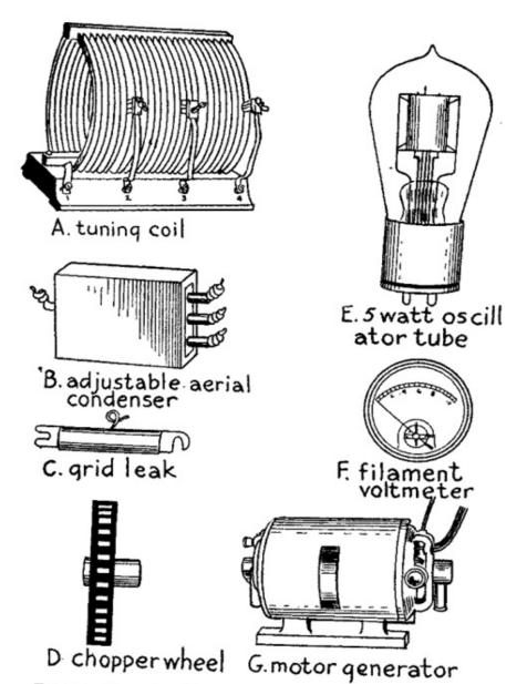
Fig. 77.—Apparatus of 100 Mile C. W. Telegraph Transmitter.
