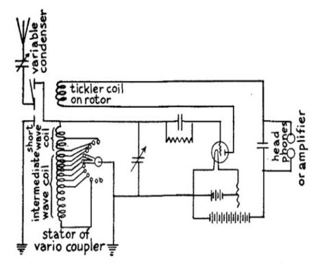
Fig. 58.—Wiring Diagram for Intermediate Wave Receptor with one Variocoupler and 12 section Bank-wound Inductance Coil.
