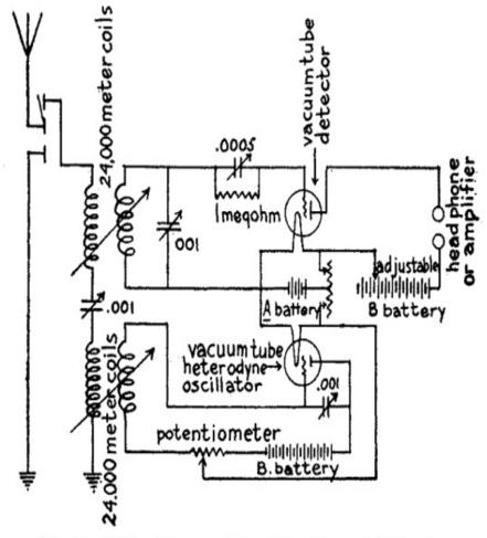
Fig. 61.—Wiring Diagram of Long Wave Separate Heterodyne Receiving Set.
