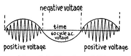
Fig. 95.—Positive Voltage only sets up Oscillations.
