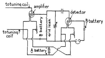
(B) Fig. 44.—Wiring Diagram for Using One A or Storage Battery with an Amplifier and a Detector Tube.
