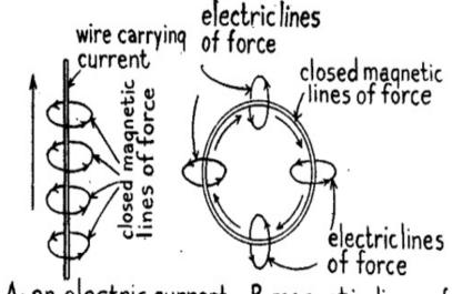
A- an electric current B-magnetic lines of force changed into electric lines of force changed into magnetic lines of force
