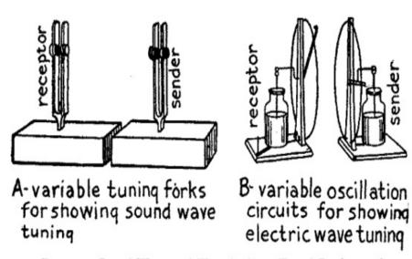
Fig. 36.—Sound Wave and Electric Wave Tuned Senders and Receptors.
