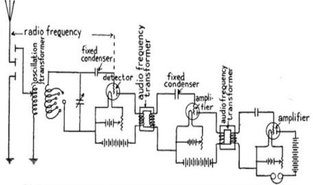
(B) Fig. 46.—Wiring Diagram for an Audio Frequency Transformer Amplifying Receiving Set. (With Vacuum Tube Detector and Two Step Amplifier Tubes.)
