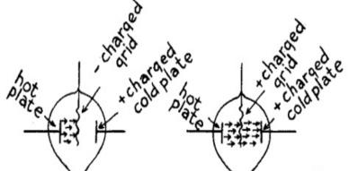
A. a negatively charged B. a positively charged qrid stops the qrid lets the electrons pass
