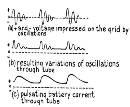
(D) Fig. 72.—How the Oscillations Control the Flow of the Battery Current through the Tube.
