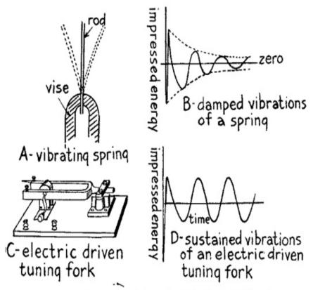
Fig. 34.—Damped and Sustained Mechanical Vibrations.
