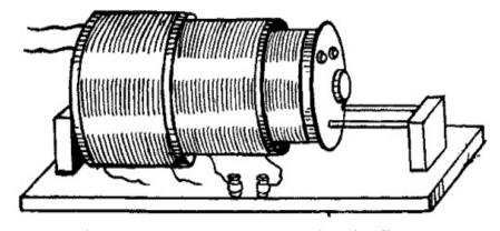
(B) Fig. 49.—Three Coil Loose Coupler Tuner.
