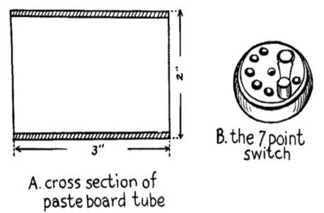
Fig. 97.—How the Tuning Coil is Made.
