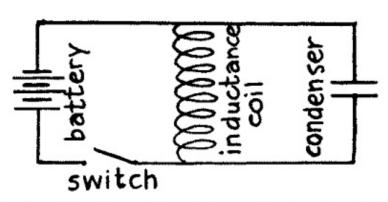
(C) Fig. 94.—How a Direct Current Sets up Oscillations.
