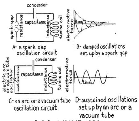
Fig. 35.—Damped and Sustained Electric Oscillations.
