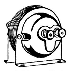
(B) Fig. 45.—Radio Frequency Transformer.
