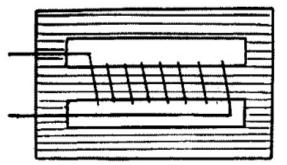
A. wiring diagram of a filter reactor
