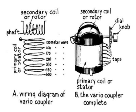
Fig. 53.-How the Variocoupler is Made and Works.
