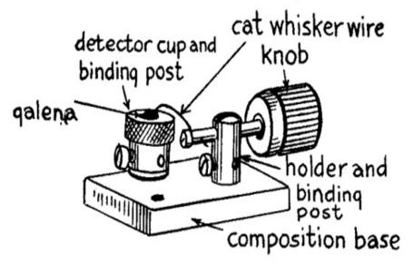
Fig. 96.—Rasco Baby Crystal Detector.
