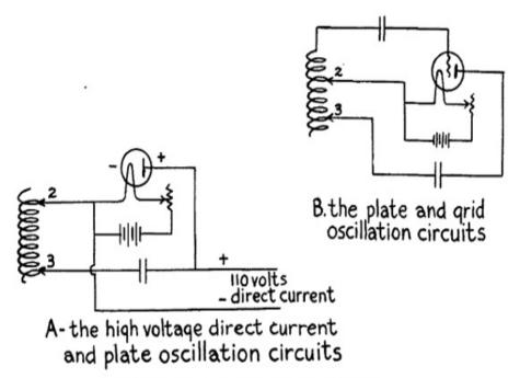
(A) and (B) Fig. 94.—Operation of Vacuum Tube Oscillators.
