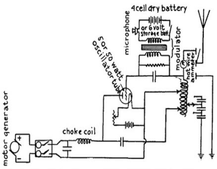
(A) Fig. 89.—Wiring Diagram of 25 to 50 Mile Wireless Telephone. (Microphone Modulator Shunted Around Grid-Leak Condenser.)
