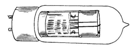
Fig. 80.-50 Watt Oscillator Vacuum Tube.
