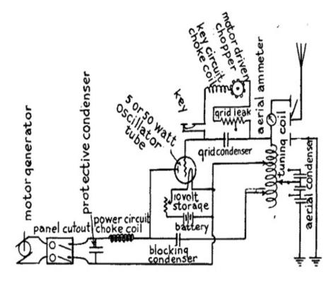
Fig. 78.—5 to 50 Watt C. W. Telegraph Transmitter. (With Single Oscillation Tube.)
