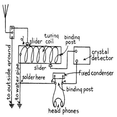
(A) Fig. 15.—Top View of Apparatus Layout for Receiving Set No. 1.
