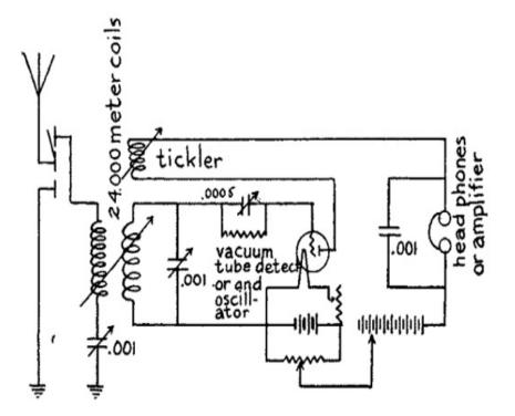
Fig. 60.—Wiring Diagram of Long Wave Antodyne, or Self-Heterodyne Receptor.
