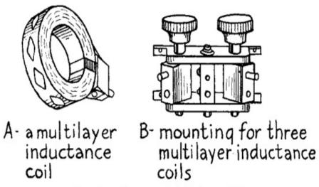
Fig. 50.—Honeycomb Inductance Coil.
