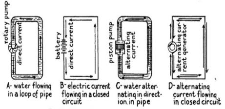
Fig. 29.-Water Analogues for Direct and Alternating Currents.
