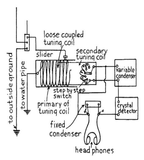
(A) Fig. 16.—Top View of Apparatus Layout for Receiving Set No. 2.
