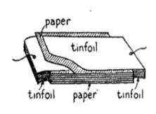
(A) Fig. 13.—How a Fixed Receiving Condenser is Built up.
