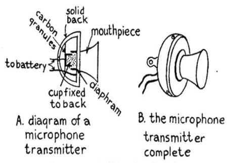
Fig. 84.—Standard Microphone Transmitter.
