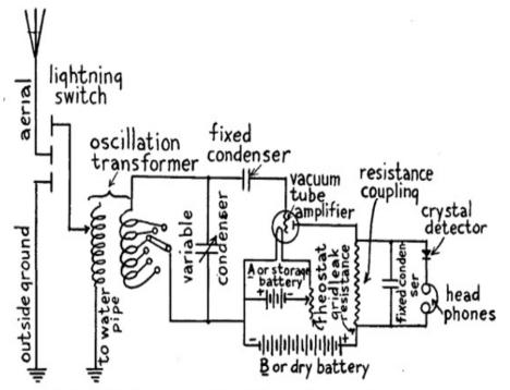
Fig. 43.—Crystal Detector Receiving Set with Vacuum Tube Amplifier (Resistance Coupled).
