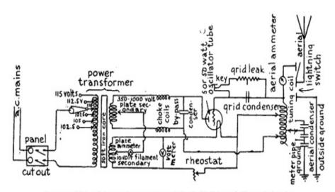
Fro. 82.—Wiring Diagram for 200 to 500 Mile C. W. Telegraph Transmitting Set. (With Alternating Current.)
