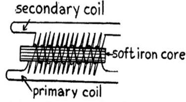
A. wiring diagram of induction coil
