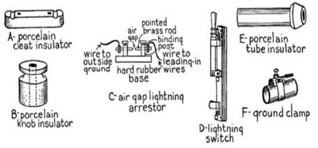
Fig. 5.—Material for a Simple Aerial Wire System.
