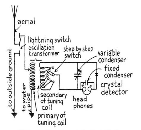
(B) Fig. 16.-Wiring Diagram for Receiving Set No. 2.
