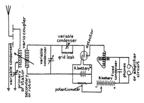
Fig. 55.-Short Wave Regenerative Receiving Set (one Variometer and three Variable Condensers.)
