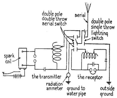
Fig. 26.—Wiring Diagram for Complete Sending and Receiving Set No. 1.
