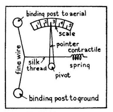
Fig. 24.—Principle of the Hot Wire Ammeter.
