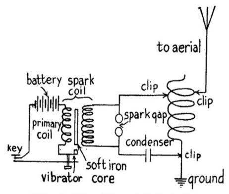
(B) Fig. 20.—Wiring of Diagram for Sending Set No. 1.
