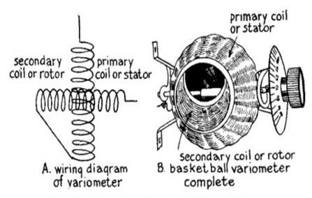
Fig. 54.—How the Variometer is Made and Works.
