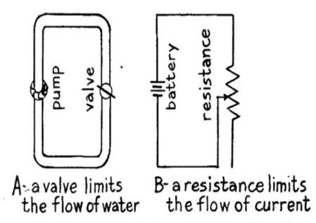
Fig. 31.—Water Valve Analogue of Electric Resistance.
