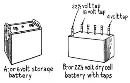
Fig. 39.—A and B Batteries for Vacuum Tube Detectors.
