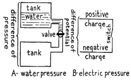
Fig. 28.—Water Analogue for Electric Pressure.
