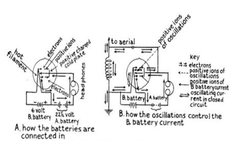
(A) and (B) Fig. 71.—How a Two Electrode Tube Acts as a Relay or a Detector.
