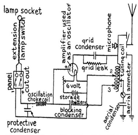
Fig. 85.—Wiring Diagram of Short Distance Wireless Telephone Set. (Microphone in Aerial Wire.)
