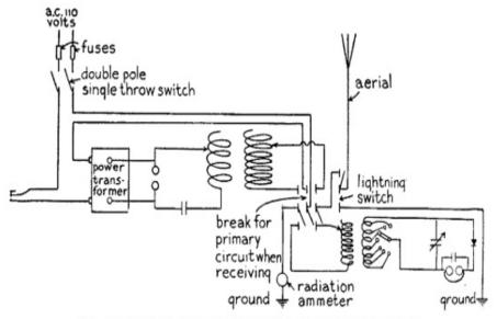
Fig. 27.—Wiring Diagram for Complete Sending and Receiving Set No. 2.
