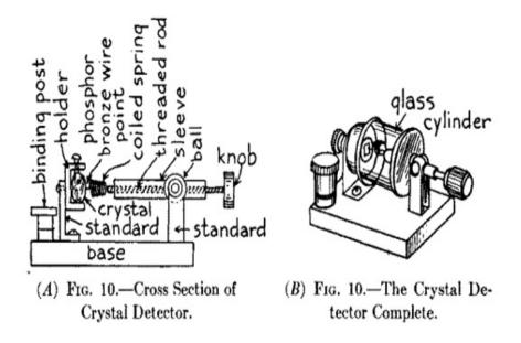
A crystal of this kind is often enclosed in a glass cylinder and this makes it retain its sensitiveness for a much longer time than if it were exposed to dust and moisture. An upright type of this detector can be bought for \$2.25, while a horizontal type, as shown at *B*, can be bought for \$2.75. Galena is the crystal that is generally used, for, while it is not quite as sensitive as silicon and iron pyrites, it is easier to obtain a sensitive piece.
