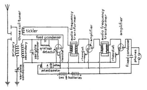
Fig. 52.—Regenerative Audio Frequency Amplifier Receiving Set.
