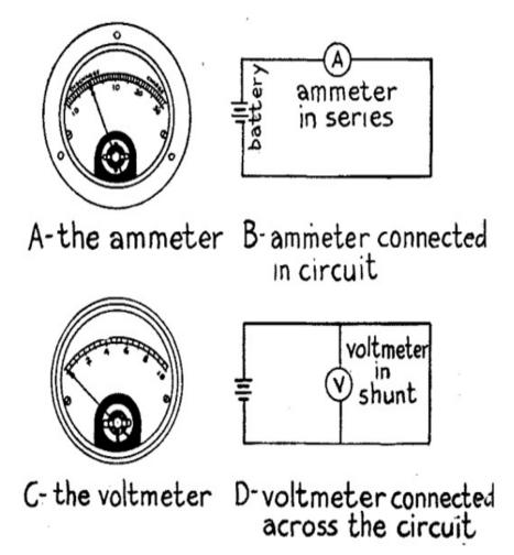
Fig. 30.—How the Ammeter and Voltmeter are Used.
