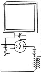
FIG.179-A SIMPLE COIL ANTENNA CIRCUIT.
