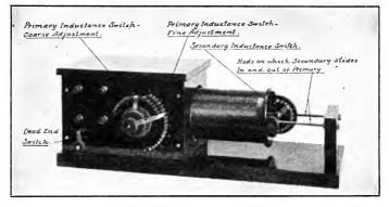
FIG. 249.-Receiving transformer.
