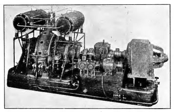
FIG. 221.-200 kw. Alexanderson alternator.
