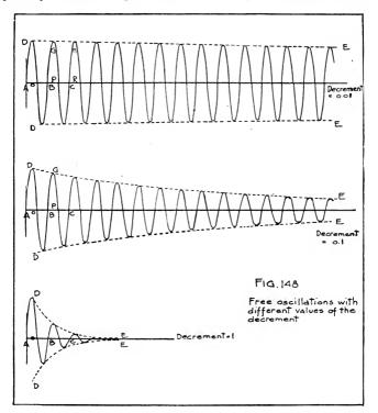
be as fully charged as at the beginning, only with the potential difference of the plates in the direction opposite to that at the start. Now begins a discharge of electricity from the condenser in the opposite direction to the first discharge, and this discharging current flows until the condenser has become fully recharged in the original direction. The cycle of operations then repeats itself, and so on, over and over again.
