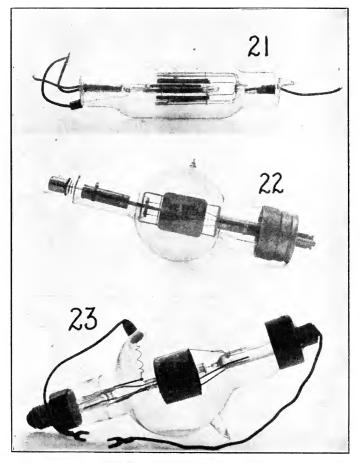
FIG. 266.—Large transmitting tubes.
