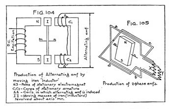
which have a very much smaller permeability than the iron conductors. The flux is consequently less. The increase and decrease of magnetic flux in the coils A A sets up an alternating emf., because any change in the flux inclosed by a circuit sets up an emf. in the circuit (Sec. 45) in the one direction while the flux is increasing, and in the opposite direction while it is decreasing.
