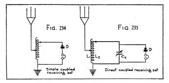
are detected by the crystal and telephone, and which are not in either oscillating circuit. The oscillations are not damped thereby, and sharp tuning is obtained.
