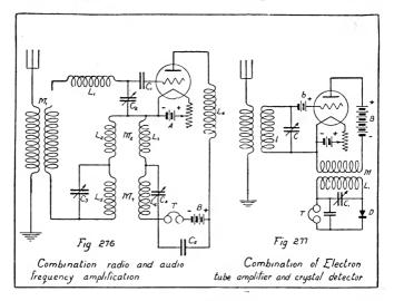
the audio frequency and of by-passing the radio frequencies. The radio-frequency variations in the plate current flow through the circuit  $PFL_{*}C_{4}C_{6}L_{4}$  and at the same time the audio-frequency variations flow through the circuit  $PFL_{*}L_{6}TBL_{4}$ . The audibility of weak signals received by this method is about 100 times the audibility obtained with a single tube connected in a simple detector circuit. On stronger signals the amplification is smaller.
