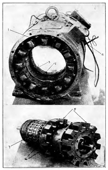
Fig. 124 .--- Inductor alternator type motor-generator set.
