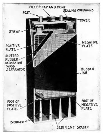
FIG. 29.-Storage cell. Lead plate-acid electrolyte type.
