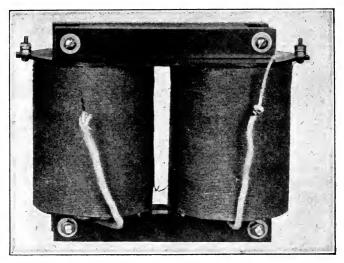
FIG. 181.—Step-up transformer for charging condenser.
