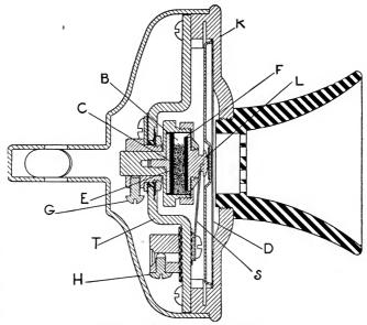
FIG. 93a.-Microphone transmitter.
