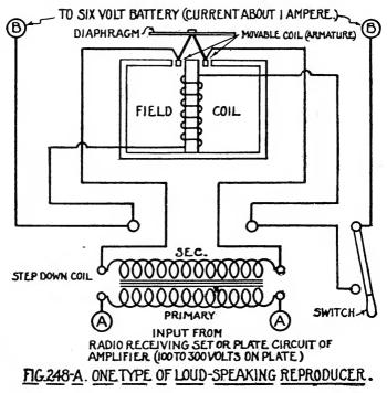
small rod to the center of the metal diaphragm, which may be aluminum. These reproducers are commonly used in connection with electron tube amplifiers of special design. (See Chap. 6.) One type of loud-speaking reproducer is shown in Fig. 248–A. The construction of one type of loud-speaking reproducer is described in United States Patents Nos. 1266988 and 1329928.
