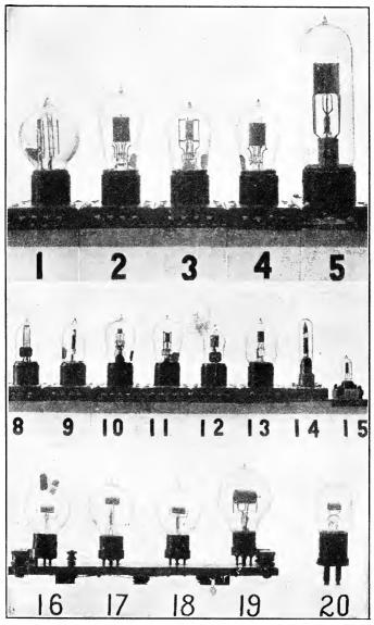
FIG. 265.—Practical forms of three-electrode electron tubes. 470
