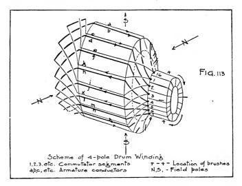
the brushes, which are thus seen to be alternately, one positive and the next negative, as we go around the commutator. If a machine having more than two sets of brushes is examined, it will be found that all the positive brushes are joined by a heavy conductor and all the negative brushes by another. Then one connection is made from the group of positive brushes to the external circuit, and one from all the negative brushes.
