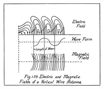
sheets have moved so far that they can be considered practically as planes, then the magnetic lines also lie in these planes, but perpendicular to the electric lines and to the direction of motion.
