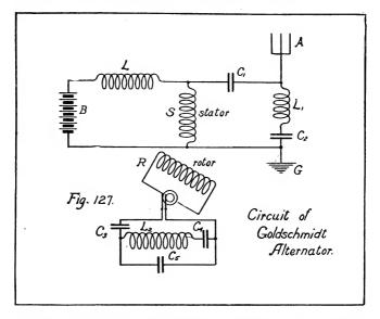
Without undertaking to give the proof here, it may be stated that when a rotor is revolved, and at the same time alternating currents are made to flow in the rotor at a frequency corresponding to the speed of rotation and to the number of poles, then, due to these currents, pulsations take place in the strength of the magnetic flux of the machine at double the frequency of the alternating currents.
