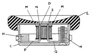
FIG. 93b.-Watch case telephone receiver.
