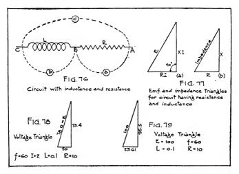
The effective applied emf. E in such a case is therefore related to the voltages RI and XI by the equation (relation between sides and hypotenuse of a right triangle),
