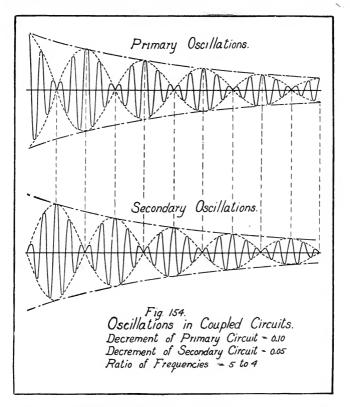
energy is entirely in the primary, at others entirely in the secondary, and at other instants partly in the primary and partly in the secondary. This transfer of energy, first in one direction and then in the other, shows that the primary and secondary play alternately the rôle of driving circuit.
