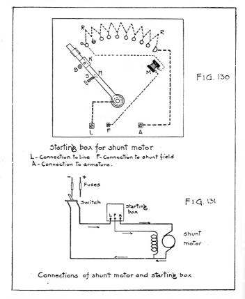
sulating face plate, commonly slate. The internal connections are drawn in dashed lines. Fig. 131 shows how the starting box is connected between the fused main switch and the motor.
