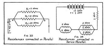
up voltage, but at the same time it increases the internal resistance, while a parallel arrangement, by decreasing the internal
