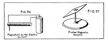
porary magnet or an "electromagnet." Examples of electromagnets are seen in induction coil and buzzer cores, in telegraph sounders and relays, and in telephone receivers. Electromagnets are very useful because the magnetism is so easily controlled by variations in the current strength. If the bars are of hardened steel, the magnetism due to the current remains after the current ceases and a permanent magnet is the result.
