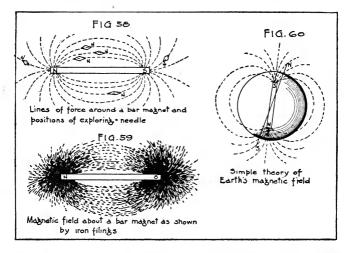
other repels the same pole, they are said to be unlike. *Like* poles repel each other and unlike poles attract each other. It is then easy to determine which is the north and which is the south pole of a bar magnet by means of the direction in which the north pole of a compass needle points.
