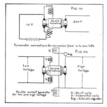
motor." An application which will occur to the radio student is the securing from batteries giving only 10 or 12 volts of the 300 or more volts required for supplying the plate potential of electron tubes used as generators of radio-frequency alternating current. (See Fig. 135.) In the dynamotor two separate armature windings are placed on a common core. One acts as a motor, the other as a generator. There is but one frame and
