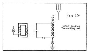
critical coupling is used. Many operators, however, fail to operate quenched gap sets properly adjusted for critical coupling. When a quenched gap is not properly adjusted, the wave may be very broad and the tone may be very poor. (See also page 360.)
