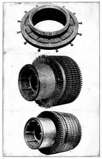
FIG. 114 (upper)—Method of assembling commutator segments. Fig. 115 (middle)—Commutator and armature core assembled showing risers. Fig. 116 (lower)—Armature complete with windings connected to risers.
