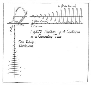
circuits in which the plate circuit is coupled back to the grid circuit in such a manner as to supply this small power to the grid and make the surplus power available for use in an external circuit in the form of continuous or undamped oscillations of any frequency from even less than one per second to 10,000,000 or more per second.
