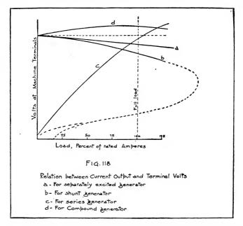
flux is weaker, the greater the armature current. Hence the terminal voltage falls off more than it does with separate excitation. Thus curve b, Fig. 118, droops more than curve a. The dashed part shows how the voltage falls off when the machine is greatly overloaded.
