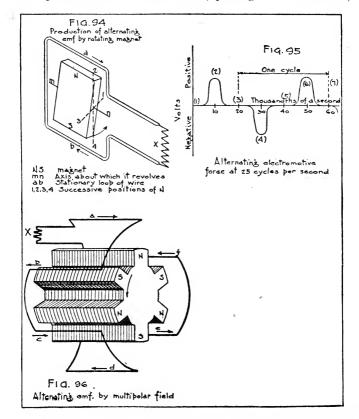
is the same as if the conductor were to move away from the reader, passing pole N.
