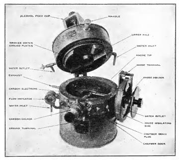
FIG. 227.-Interior of 2-kw. Federal arc converter.
