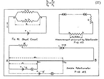
The currents in the two branches are inversely proportional to the resistances of their respective paths. This relation is called the "shunt law." In other words, it means that the branch of lower resistance carries the larger current, and the branch of higher resistance carries the smaller current.
