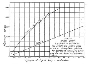
also shows for air at atmospheric pressure the maximum values of sparking voltages corresponding to various lengths of gap with terminals consisting of spheres one inch (2.54 cm.) in diameter. The results used in plotting both curves were obtained with alternating current, but will also apply to the measurement of d.c. voltages.
