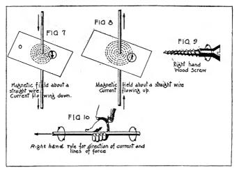
curved finger tips will then indicate the direction of the magnetic effect, Fig. 10.
