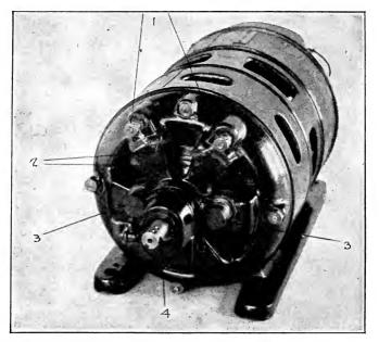
FIG. 121.—Small 500-cycle motor-generator set (2500 r.p.m.; 24 poles on stator: 24 teeth on rotor; 110 volts; 3.2 amp.; 0.35 kya.).
