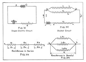
nected as shown in Fig. 34, so that only a part of the current passes through each resistance, they are said to be connected in "parallel" or "multiple." The voltage E between points a and b is the same over any branch. We may then write, from equation (11),
