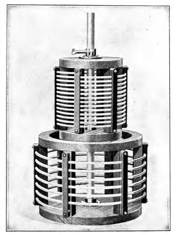
FIG. 197.—Double helix oscillation transformer; coils separated axially. cuited except when actually needed in order to keep the resistance of the antenna circuit low.
