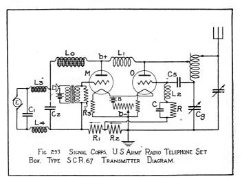
be maintained as in land telephony without throwing an antenna switch from transmitter to receiver. In these sets means are provided so that an outgoing message will not greatly affect the receiver phones, while an incoming message will.
