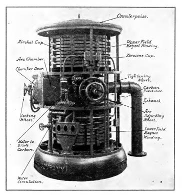
FIG. 226.—100-kw. Federal arc converter, with casing removed.
