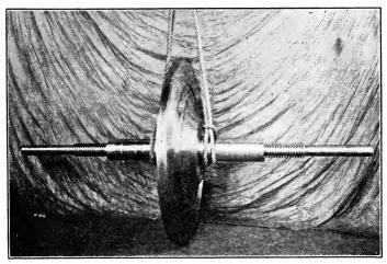
FIG. 126c.-Rotor of 200 kw. Alexanderson alternator.
