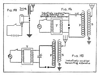
connecting the current source across the gap. Arcing in the gap must be guarded against, and care should be taken not to open the gap too wide, or the antenna insulation may break down.
