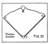
ends are connected by a copper wire through the galvanometer g. If the point of contact, or junction J, is heated to a temperature above that of C and C', there will be a flow of current through the galvanometer. This is commonly explained by saying that at the junction J, heat energy is transformed into electrical energy, and this
