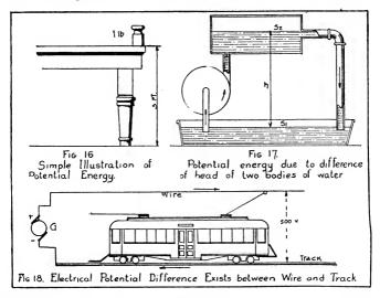
amount of potential energy possessed by a body when placed there. In other words, a body placed at this point is able, by virtue of its position, to do a certain amount of work. If we assume that the body has unit mass, this characteristic is called the gravitational potential of the point. The higher position is said to have a higher potential than the lower position, and the difference in potential, measured in terms of work, is a measure of the difference in height.
