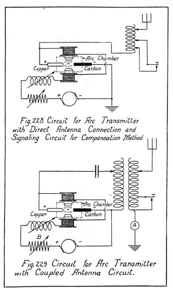
ductances in series with the antenna. The connections of a typical arc transmitter of American manufacture are shown in Fig. 228. In some types of arcs of European manufacture the antenna circuit is coupled as shown in Fig. 229. The antenna loading coils are usually wound with stranded high-frequency conductor to minimize the high-frequency resistance. (See Sec. 117.)
