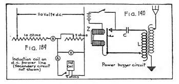
first attempt to signal, and the current will not be broken when the key is released. Of course, the method of inserting a rheostat is very wasteful, since the  $RI^2$  loss in the rheostat is large, much greater in fact, than the power actually used in the radio apparatus.
