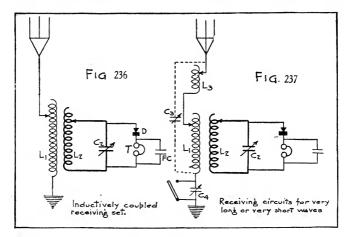
rent are filled in, and the cumulative effect of a wave group is strengthened. In practice the telephone cord, containing as it does two conductors separated by dielectric, forms a condenser which in some cases is sufficient so that an added fixed condenser gives no improvement.
