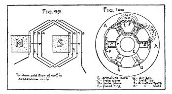
resultant electromotive force begins to decrease, falling to zero and then beginning to increase in the opposite direction. In this manner an alternating emf. is gotten in which the changes occur gradually as conductors get into or out of the magnetic field one by one, or at least coil by coil. In addition the edges of the poles are usually tapered off ("chamfered") to make the changes still smoother.
