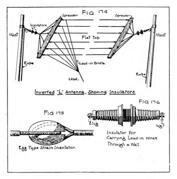
better insulation when the insulator is wet by collecting the water on the lowest points of the ribs. In the case of antennas for land stations, wire guys are interrupted by "strain" insulators to prevent the guy from having a natural wave length approximately the same as the wave length of the antenna. A form of nearly spherical porcelain insulator, so grooved as to carry the two wires firmly without their coming in contact, is
