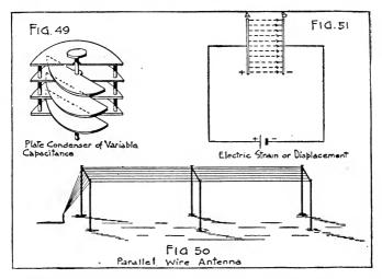
can be calibrated so that the capacity corresponding to any angular setting of the rotating part is known. Condensers used in radio circuits are represented by certain symbols. These symbols may be found in Appendix 3, page 553.
