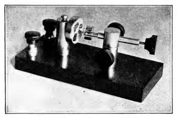
FIG. 245.—One method of mounting crystal detectors.
