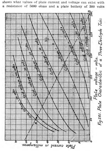
externally placed between the filament and plate of the tube. If the grid voltage, for example, is -10, then the plate voltage will be 220 volts and the plate current 16 milliamperes, as de-
