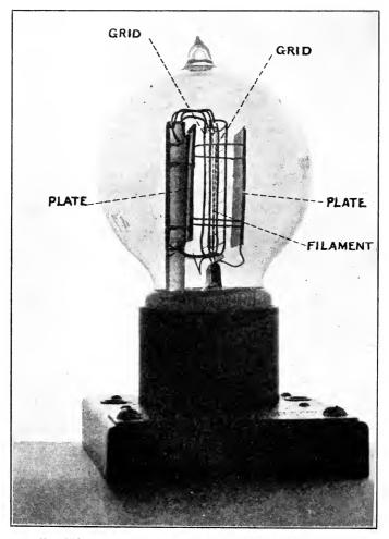
FIG. 256.—Construction of the three-electrode electron tube.
