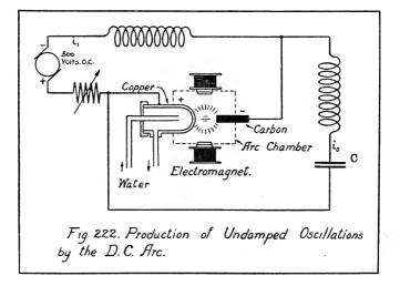
a pulsating d.c. voltage is applied to the arc, the a.c. component of the current will be  $180^{\circ}$  out of phase with the a.c. component of voltage.
