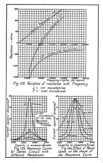
quency are the same and have the value 316.2 ohms. This value may, of course, be calculated by using for f the value of the resonance frequency in either of the expressions  $2\pi fL$  or  $\frac{1}{2\pi fC}$ . It is of interest to note that each of these expressions for reactance reduces simply to  $\sqrt{\frac{L}{C}}$ , when the frequency has the resonance value.
