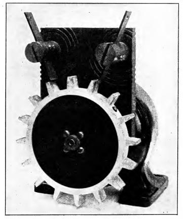
FIG. 186.-Nonsynchronous rotary gap.
