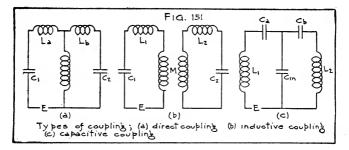
tive reactance is appreciable at radio frequencies, and in this case the effect of the coupled coils is a combination of inductive coupling and capacitive coupling.
