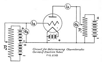
acteristics for a tube used in receiving equipment, this being obtained (see Fig. 258) by setting the plate voltage at 20, 40, 60 volts in turn and finding how the plate current changes as the grid voltage is changed. Fig. 260 shows the grid current determined under the same conditions. An alternate method of expressing characteristics is shown in Figs. 261 and 262.
