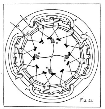
FIG. 125.—Self-excited inductor type alternator. (4500 r.p.m.; 75 volts; 5 amp., 900 cycles per second.) A, terminals of a.c. winding;
