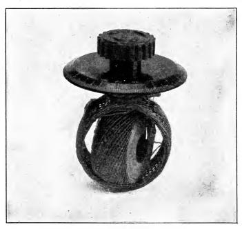
FIG. 250.-Lattice-wound variable coupling coil.
