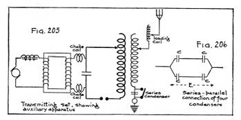
levers, changes simultaneously the adjustments on all three coils. From these coils are taken out taps over which three switch blades pass, adjusting all the inductances to approximately the values needed for the particular wave length desired, keeping the circuits in resonance and at the proper coupling. For fine adjustments an additional variable inductor may be provided in the primary and in the secondary.
