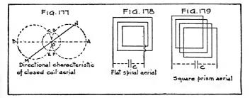
its natural wave length. That is, to receive short waves a coil of small inductance and small distributed capacity should be used. Such a coil must have few turns. To receive longer waves, coils of a larger number of turns may be used. Experience shows that best results are obtained with one or two turns embracing a large area for use with short waves, and for long waves coils with 20 to 30 turns, or even 100 turns, not so large in area.
