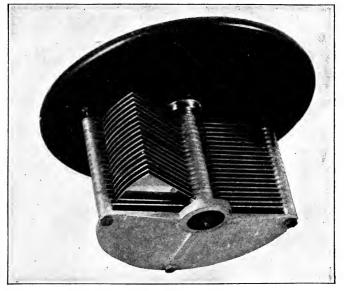
FIG. 251.-Rotary variable air condenser.
