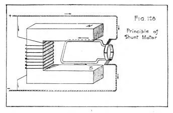
to make the rotation continuous by making the proper connection to the conductors as they come into place.
