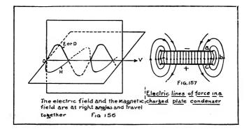
(b) The magnetic field intensity resulting from the displacement current is at right angles to the displacement and to the direction of the wave train.
