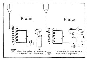
The two-electrode electron tube is now practically obsolete as a detector. Present practice is to use a three-electrode tube.
