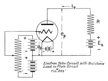
tube is used for producing a magnified output, whether the tube is used as a detector, amplifier, generator, or modulator. In receiving tubes the variations of tube quantities are small compared with average values, but in transmitting tubes they are large.
