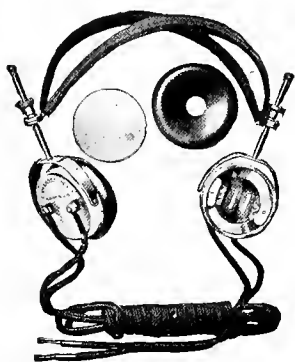
FIG. 127.—Telephone receivers, or, as they are also called, the head-set.
