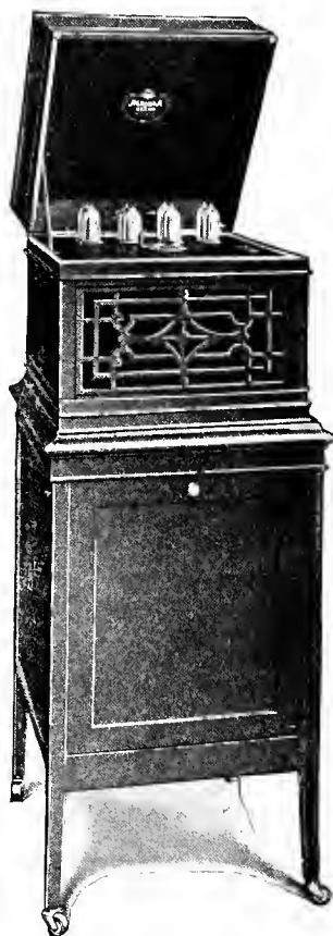
FIG. 139.—De Luxe receiving set designed by the Westinghouse Company. Single circuit regenerative set with 3 stages audio-frequency amplification. Filaments of tubes regulated by ballast tubes instead of rheostats. Loud speaker contained in cabinet.
