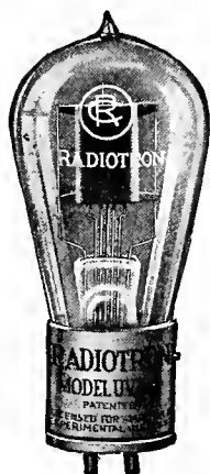
FIG. 146.—Five Watt transmitting tube for use in transmitters, such as shown in Figures 143 and 145.
