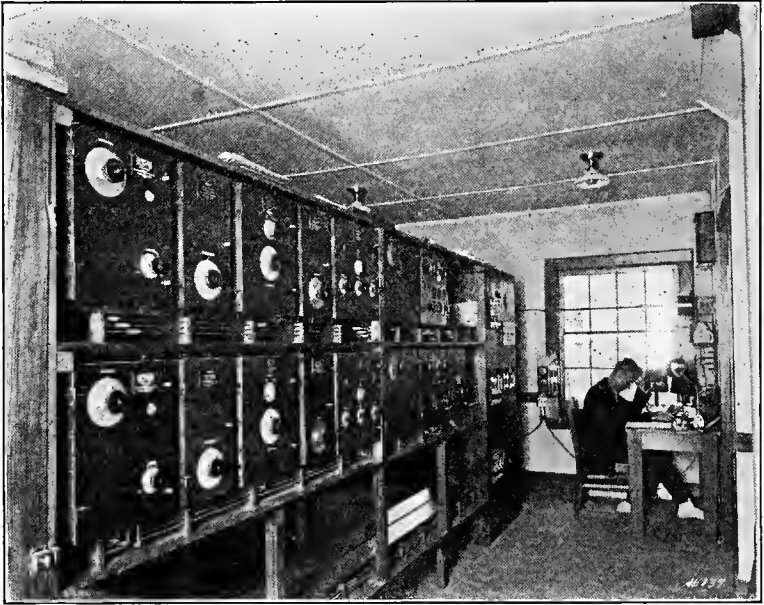
FIG. 180.—Each of the two shelves in this photograph contains a complete receiving set for receiving radio telegraph messages from Europe. This is part of the trans-Atlantic receiving station of the Radio Corporation, located at Riverhead, L. I.
