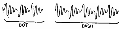
FIG. 35.—A transmitting station sends out the letter A, by pressing the key for a short interval, and then for a longer interval, closing the circuit for a corresponding length of time and causing, first, a short series of oscillations to be radiated and then a longer series. These are respectively a dot and dash.
