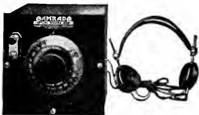
FIG. 68.—A compact portable crystal receiving set manufactured by American Radio and Research Company.
