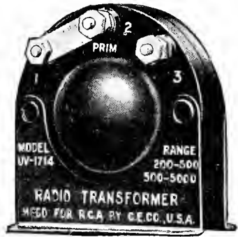
FIG. 103.—Radio frequency transformer. The shunt shown at the top of the transformer can be changed so that either a range of from 200 to 500 meters, or from 500 to 5000 meters are available.
