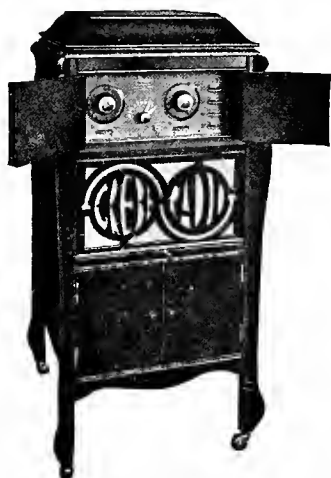
FIG. 138.—De luxe receiving set containing single circuit regenerative receiver, detector, three stages of audio-frequency amplification, and loud speaker. This makes an almost ideal type of apparatus for home entertainment.
