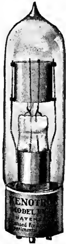
FIG. 144. — Keno-tron rectifying tube for use in transmitting circuits where only A.C. is available.
