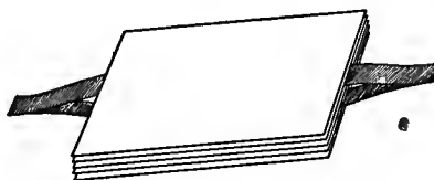
FIG. 44.—Fixed condenser assembled.
