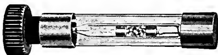
FIG. 61.—Mineral detector in a vacuum, which protects the mineral. Adjustment is made by turning knob.
