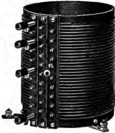
FIG. 81.—Transmitting tuning coil arranged with plugs for changing wave length.
