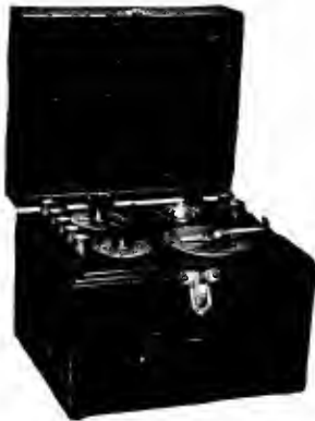
FIG. 165-A.—Westinghouse single circuit vacuum tube receiver which operates on one dry cell.
