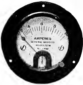
FIG. 88.—Hot-wire ammeter, to be connected in series with aerial, to show the amount of current that is being delivered to it.
