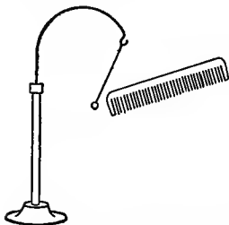
FIG. 4.—Like charges of electricity repulse each other.
