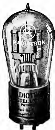
FIG. 107.—Vacuum tube for a receiving set.
