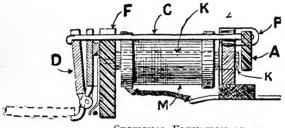
SECTIONAL ELEVATION AT x.y. Fig. 43 TWO-COIL DROP (FULL SIZE)
