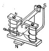
Fig. 15 principle of siemens polarized relay
