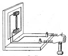
Fig. 38 HUGHES'S "PENCIL" MICROPHONE CONNECTIONS
