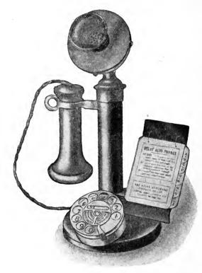
Fig. 51 TABLE SET FOR AUTOMATIC WORKING
