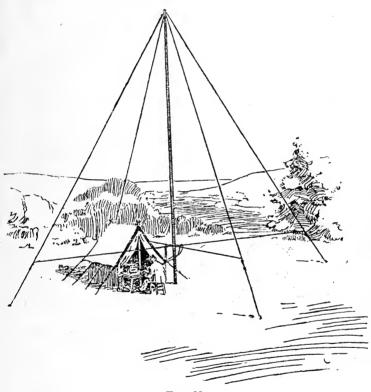
FIG. 68 MARCONI DIRECTION FINDING STATION
