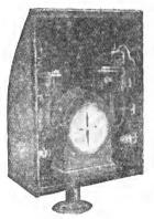
FIG. 23 POLARIZED DOUBLE-PLATE SOUNDER
