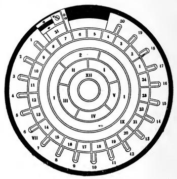
Fig. 28 BAUDÔT MULTIPLEX FRONT PLATE RINGS AND SEGMENTS
