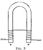
CORRECT METHOD OF WINDING ELECTRO-MAGNET.
