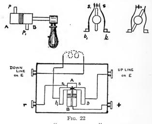
CONNECTIONS OF "DROP-HANDLE" SINGLE NEEDLE
