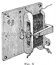
FIG. 5 CONSTRUCTION OF DETECTOR GALVANOMETER
