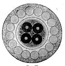
Fig. 57 SECTION OF ANGLO-BELGIAN SUBMARINE CABLE (FULL SIZE)
