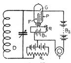
Ftg. 67 THREE-ELECTRODE THERMIONIC VALVE AMPLIFYING CIRCUIT
