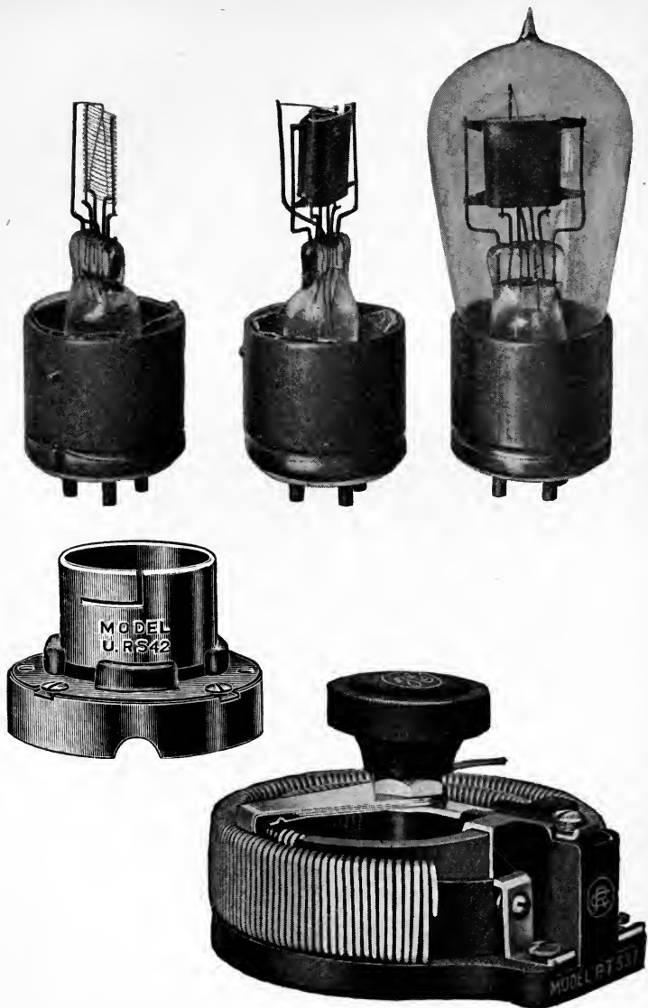
Plate V.—Above: Vacuum tube for detection; below: Tube socket and filament rheostat; Radio Corporation of America.
