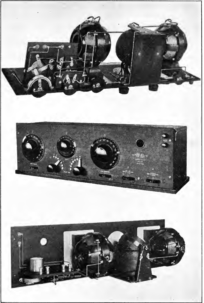
Plate VIII.—Regenerative short-wave receiving set (exterior and interior); A. H. Grebe & Company.
