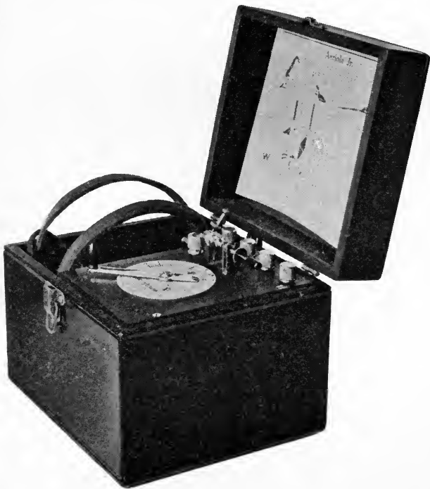
Plate IV.— Above: Crystal detector; Wireless Specialty Apparatus Company . Below: “Aeriola, Jr.,” crystal-detector receiving set; Westinghouse Electric & Manufacturing Co.
