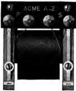
Type A-2 Acme Amplifying Transformer
