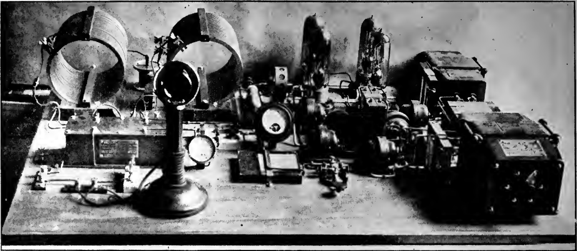
This is a highly refined vacuum tube transmitter circuit, such as is used for instructional and experimental purposes in colleges and laboratories. Completely wired, as this set is, it would be a valuable asset for any dealer, helping him to sell units
