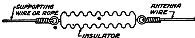
FIG. 23. The insulator is used to prevent the electrical energy leaking off the antenna to the ground through the antenna supports.
