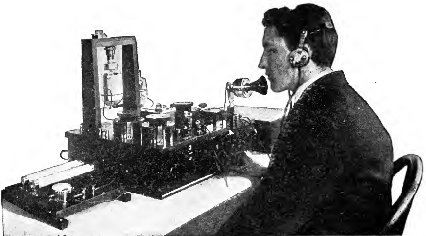
Fig. 325B—Oscillating Valve Wireless Telephone Set Developed by Marconi's Wireless Telegraph Co., Ltd.
