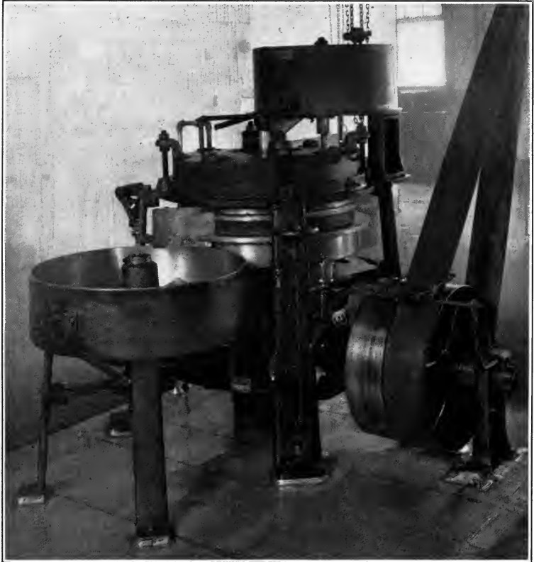
FIGURE 9.—STONE MILL FOR GRINDING INK WHERE A GREAT DEGREE OF FINENESS IS NOT REQUIRED.
