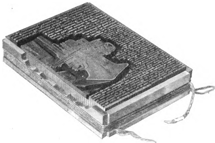
FIG. 132.—Showing Monotype Method of Mounting Cut Directly on Quads, and also Form and Use of Tie-up Slugs.
