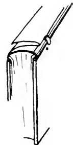
Fig.33. Folded paper for hollow back cover.
