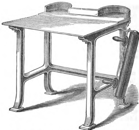
BRAYER INKING TABLE, WITH ROLLER.
