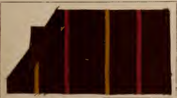
Dyed with: 3% Benzo Chrome Brown B; discharged with: 3% Rhodamine 6G, Persian berry Yellow discharge.
