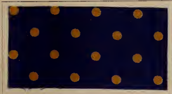
Dyed with: 3% Benzo Blue RW (coppered); discharged with: Persian berry Yellow discharge.
