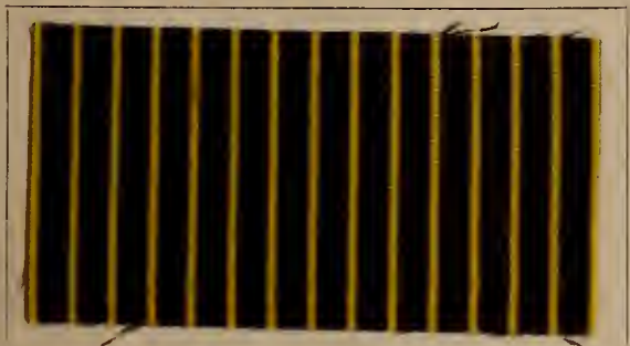
Alizarine Bordeaux BP and Chrysophenine discharged with chlorate of soda.
