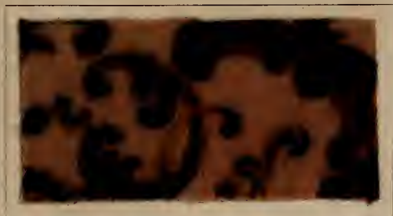
Dyed with: Benzo Purpurine 4 B; discharged with: Persian Berry Yellow and Methyl Violet.
