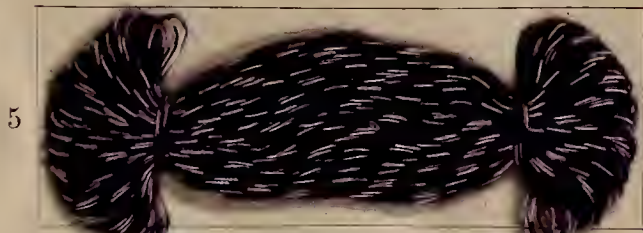
Dyed with: 5% Benzo Violet R; discharged with: tin crystals discharge.
