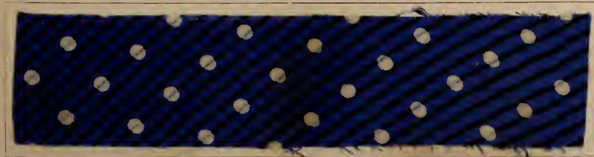
Dyed with: 2% Brilliant Azurine 5 G; discharged with tin, and cover printed with Aniline Black.
