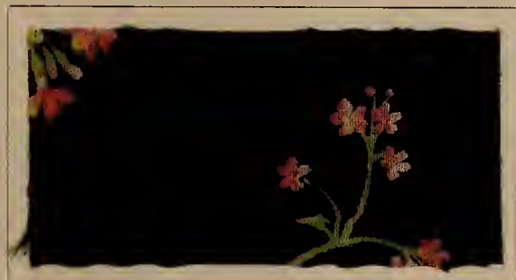
Aniline Black discharged with Brilliant Geranine B, Benzo Purpurine 4 B, Chrysophenine; Benzo Sky Blue and Chrysophenine (Olive) and afterwards mercerised.
