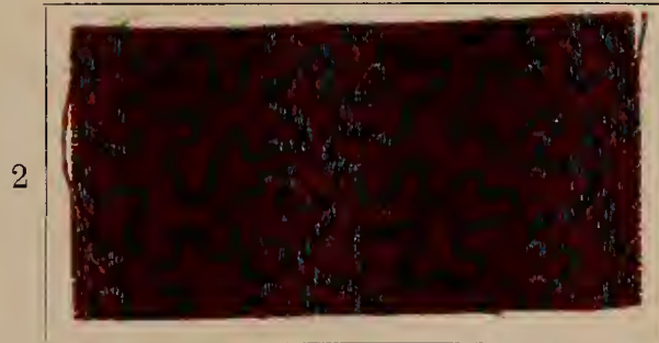
Dyed with: 2% Benzo Chrome Brown R; discharged with: 1½% Methylene Blue B B.
