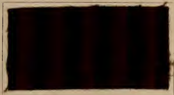
Aniline Black; dyed with 3% Benzo Nitrol Brouw G and afterwards treated with Paranitraniline.
