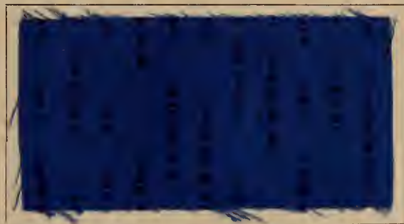
Dyed with: 2% Brilliant Benzo Blue 6 B. Cover printed with: 1/2% Diamond Fuchsine.
