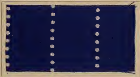
Dyed with: 3% Benzo Cyanine B; discharged with zinc powder.
