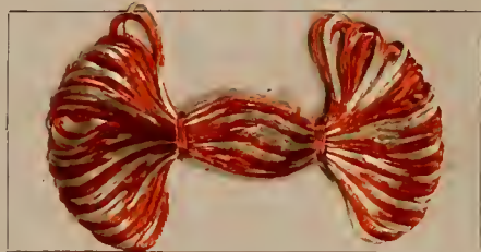
Dyed with: 4% Benzo Purpurine 1 B; Discharged with: zinc powder.
