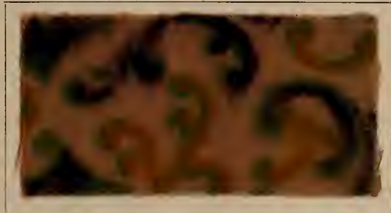
Dyed with: Benzo Purpurine 1 B; discharged with: Methyl Violet, Brilliant Green, Persian Berry Yellow.
