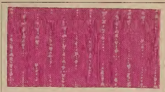
Dyed with: 0.5% Brilliant Geranine B; Printed with: zinc white.
