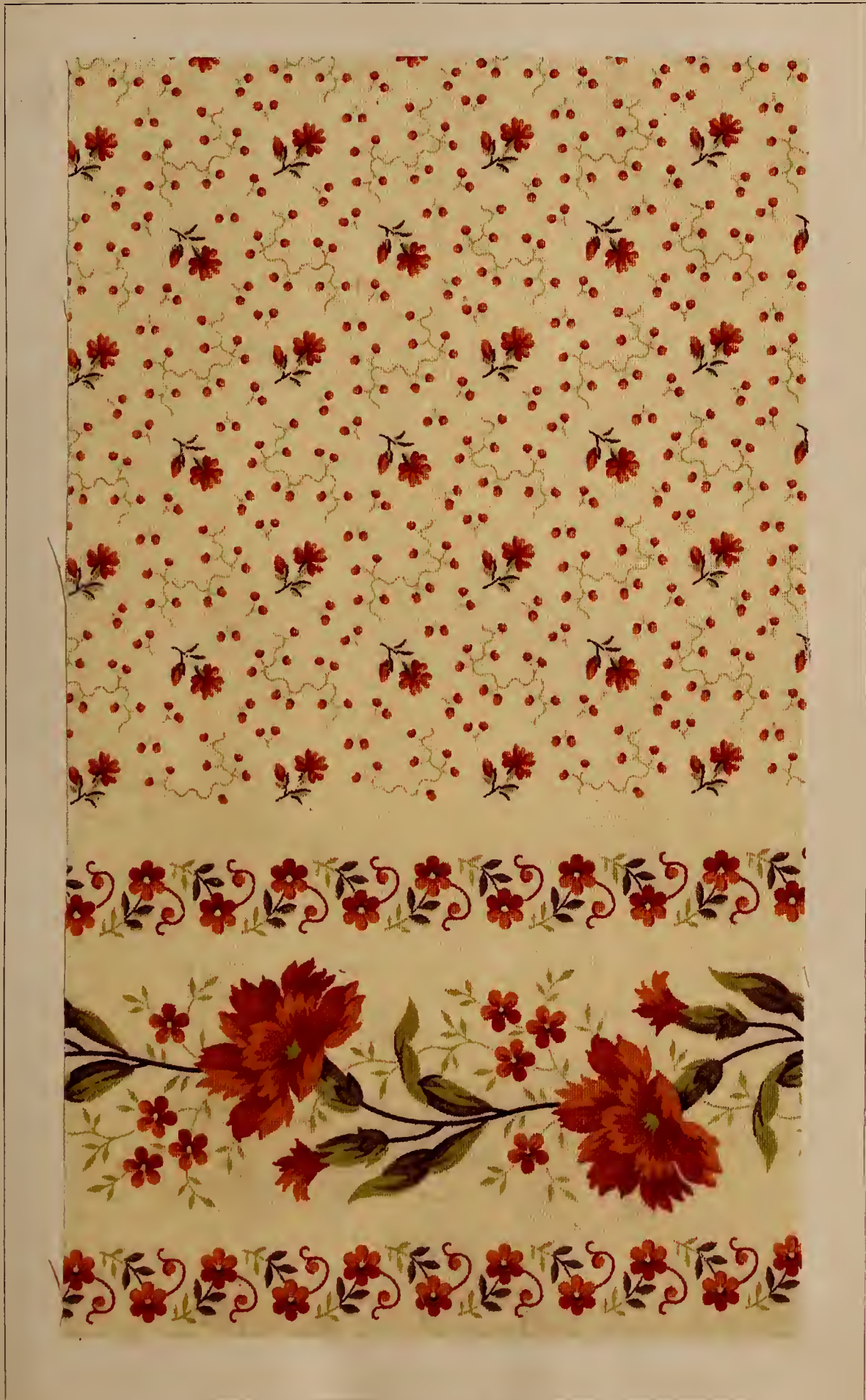
Printed with Steam Colours: finished with Chrysamine G.
