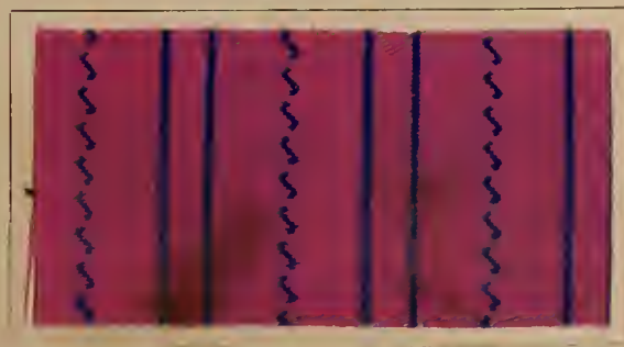
Dyed with: 1% Geranine G. Cover printed with: 1% Methylene Blue B B.
