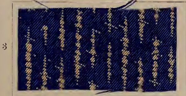
Dyed with: Brilliant Benzo Blue 6 B; Discharged with: zinc powder.
