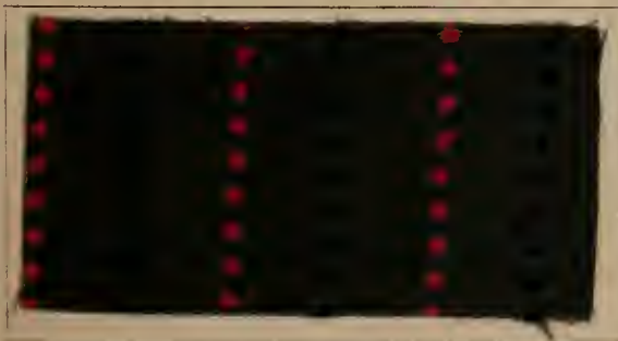
Dyed with: 3% Benzo Green G; discharged with: 3% Rhodamine 6G; printed with: 30% Fast Black.
