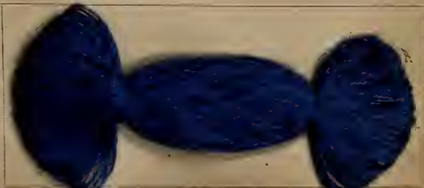
Printed with: Caustic Soda; Dyed with: 2% Brilliant Benzo Blue 6 B.
