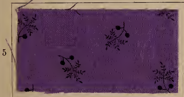
Aniline Black; dyed with 1% Heliotrope B B.
