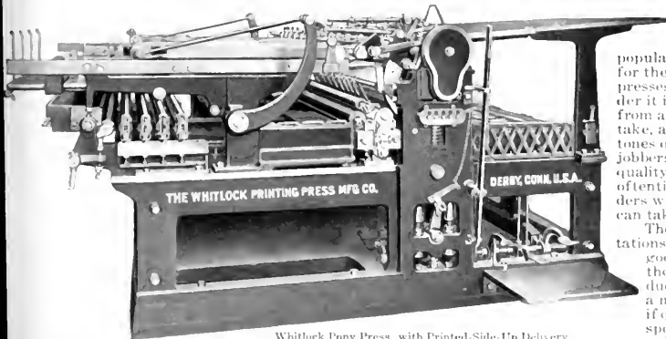
Whitlock Pony Press, with Printed-Side-Up Delivery
