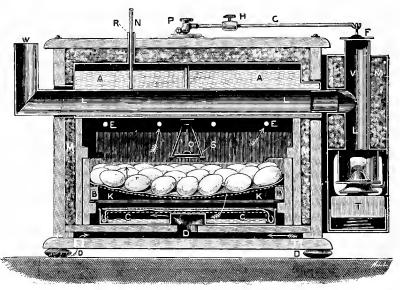
Fig. 35.-A Tank Incubator (Hearson's Pattern).
