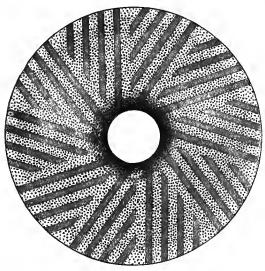
Fig. 66.-Stone Dressed for Grinding Oats.
