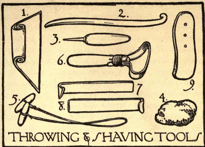
FIG. 27. 1, "Rib"; 2, Modelling Tools; 3, Pricker; 4, Sponge; 5, Wire; 6, 7, and 8, Shaving Tools; 9, Leather.
