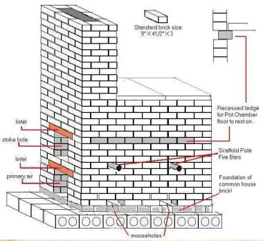
This is a drawing of the brick chimney'd kiln as it evolved before the perforated floor version; useful for brick counting and with some detail notes as well.
