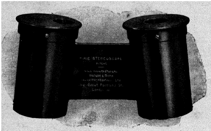
FIG. 188.—THE PIRIE STEREOSCOPE FOR X-RAY EXAMINATION.
