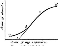
Fig. 4. - A Typical H. & D. Curve
