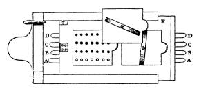
over it. The openings in this moveable plate are parallel to each other. They are seven in number, each opening being one-half of the following one, and double that of the preceding one. Thus, after the operation of the light, we have seven separate images, the different intensities of which represent the action of light during the intervals of time in the geometric progression of—1:2:4:8:16:32:64.
