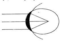
effected. A meniscus lens, therefore, with a convex surface, part of an ellipsoid, the focal distance of which coincides with its farther focus, and a concave surface, part of a sphere, whose centre is that focus, will meet all our requirements. The mecha-
