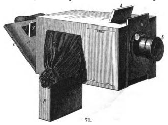
sleeves c. The yellow glass window which admits light into the camera during an operation is under the door h. i is the sliding frame for holding the focussing glass, or the frame with the
