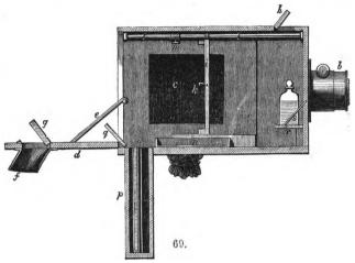
This opening is closed, when necessary, by the door g, which can be opened by the hand passed into the camera through the
