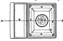
of iodine are prevented from rising and staining the plate, while the vapour, of course, passes freely through it. E is the board with the plate attached, which rests on the four smaller projecting pieces, F, fig. 5. c is the lid of the box, which is kept closed, except when the plate is
