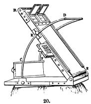
which is fixed in an independent frame, as shewn in Figs. 21 and 22, and as placed in its position at F in the adjoining cut. A black silk webbing being fixed to the moveable plate seen at the head of the instrument, and strained over two rollers, R, R, it will be evident that the sensitive plate is screened from light until the moveable slide falling down the inclined plane passes
