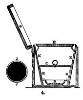
and 5, be provided. Figure 4 represents a section, supposed to pass down the middle of the apparatus by the line AB in fig. 5, which represents the box as seen from above. c is a small lid which accurately fits the interior, and divides the boxes into two chambers. It is kept constantly in its place when the box is not in use; the purpose of it being to concentrate the vapour of the iodine, that it may act more readily upon the plate when it is exposed to it. the little capsule in which the
