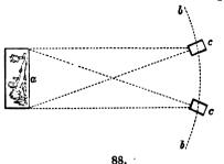
feet from the point a: the picture from this point being taken, the camera is moved round, still preserving the same distance from the object by means of a cord attached to the camera obscura, or by measuring the space. Two cameras with lenses of the same focal length
