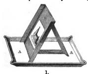
board, B, fixed at a large angle, in the trough A A, the supports being joined to it by hinges, to admit of the necessary changes of inclination, under different circumstances: two small blocks, not thicker than the tablet, are fixed on the board, on which the plate rests. Water must now be slowly poured upon the upper part of the
