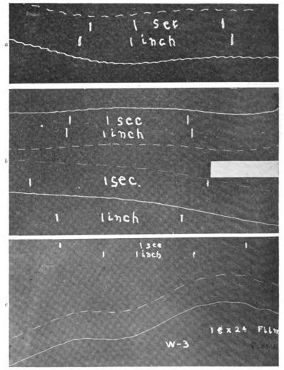
Fig. 89.—Tests of camera mountings: (a) deRam camera on bell-crank-and-spring mount, below the center of gravity; (b) same, at center of gravity; (c) type "K" film camera on universal mounting (Fig. 88).
