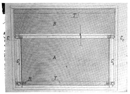
Fig. 29.—Mechanism of Klopcic variable aperture self-capping shutter.
