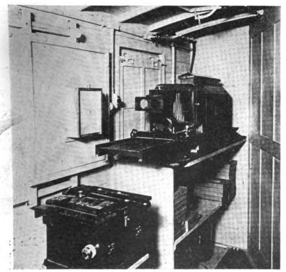
Fig. 115.—Interior of photographic trailer. Enlarging camera and printer.
