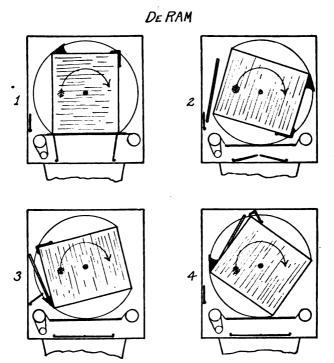
Fig. 52.—Diagram of automatic plate camera movements.
