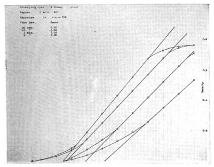
Fig. 111.-Characteristic curves of gas-light paper.
