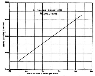
Fig. 67.—Relation between air speed and propeller revolutions.
