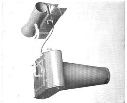
Fig. 64.—U. S. Type "K" (Folmer) automatic film canters, with wind turbine Fig. 63.—Type "K" camers, open, showing suction plate, and Venturi tube.
