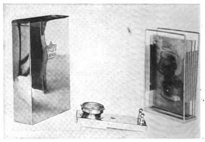
Fig. 116.—Tank and rack for tank development.
