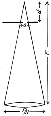
Fig. 21.—Calculation of focal plane shutter efficiency.
