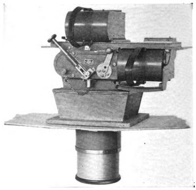
Fig. 82.-"L" camera in floor mounting.
