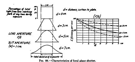
cameras, where d=4 centimeters, E=60 per cent. for the aperture assumed, which is representative. Fig. 22 exhibits diagrammatically the chief characteristics of the focal plane shutter.
