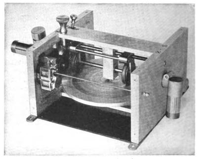
Fig. 68.—Friction disc speed control.
