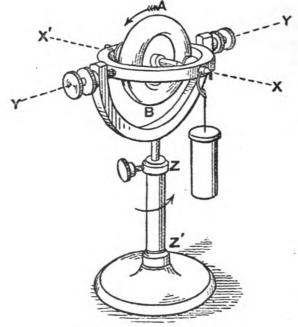
Fig. 79.—Diagram of simple gyroscope.
