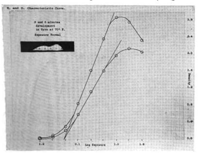
Fig. 103.—Typical characteristic curves of photographic plate.
