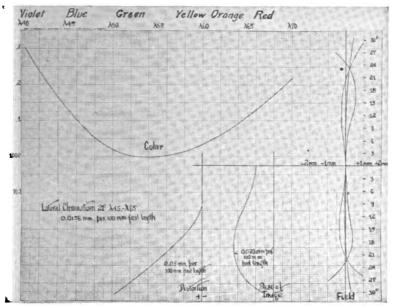
Fig. 16.—Chart recording measurements of lens characteristics.
