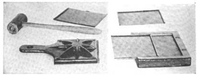
Fig. 35.—Apparatus for straightening plate sheaths.
