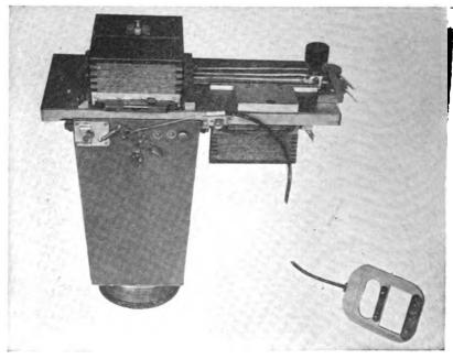
Fig. 46.—English type "E" hand-operated plate camera.
