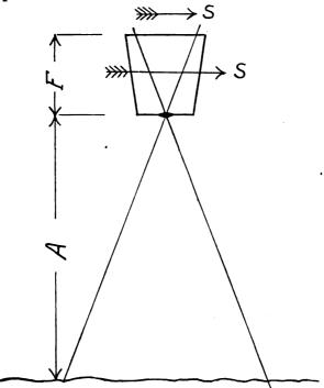
Fig. 19.—Relative motion of plane and photographic image.
