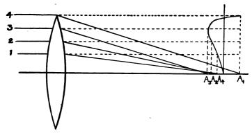
Fig. 12.—Diagrammatic representation of spherical aberration.
