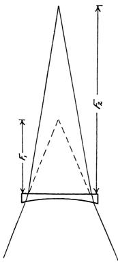
Fig. 71.—Diagram of negative lens sight.
