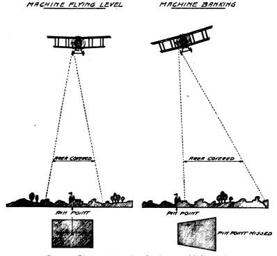
Fig. 134.—Diagram showing effect of banking on aerial photograph.
