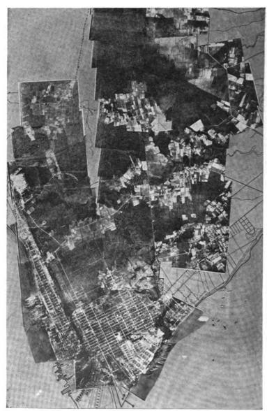
Fig. 145.—A partly completed map. Prints mounted over an outline sketch map to proper scale.
