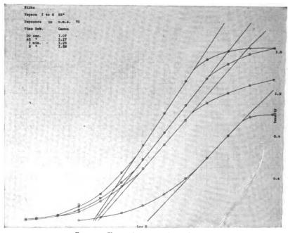
Fig. 110.—Characteristic curves of bromide paper.
