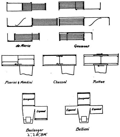
Fig. 32.—Various plate magazines used on serial cameras.
