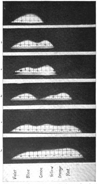
Fig. 105.—Spectrograms of representative photographic plates: a, ordinary plate; b, orthochromatic plate; c, specially green-sensitive plate; d, red sensitive plate, insensitve to green; e, panchromatic plate; f, specially red-sensitive panchromatic plate.
