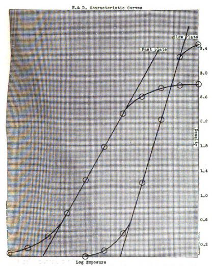
Fig. 104.—Characteristic curves of fast and slow plates, developed to maximum contrast.
