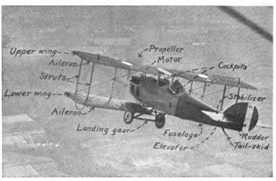
Fig. 1.-The elements of the plane.
