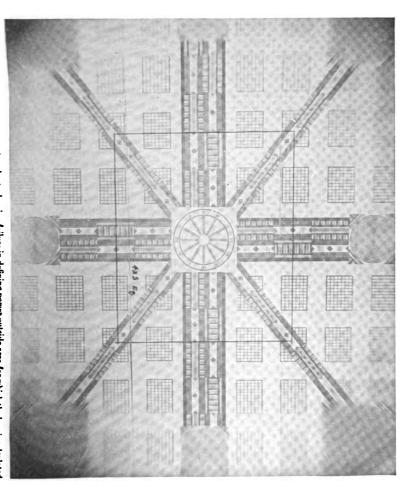
At the sides and corners the concentric circles show the lens's astigmatism, by the clear definition of the lines radial to the center of the field and their blurring in the tangential direction. The falling off in illumination with increasing distance from the center is also exhibited; and the blurring of all detail outside the rectangle for which the lens was calculated shows that spherical, chromatic, and other aberrations have become prohibitively large.
