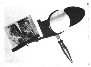
Fig. 150.—Common form of prism stereoscope.
