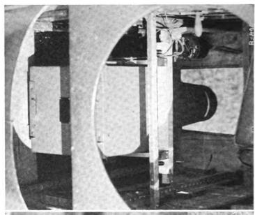
Fig. 91.—U. S. deRam camera and mount installed in photographic deHaviland 4 (Fig. 100). Viewed from above the observer's cockpit.
