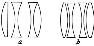
Fig. 14.—Arrangement of elements in two lenses suitable for aerial work: a, Zeiss Tessar; two simple and one cemented components (unsymmetrical); b, Hawk-eye Aerial; two positive elements of heavy barium crown, two negative of barium flint, uncemented (symmetrical).
