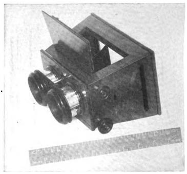
Fig. 151.—Box stereoscope.
