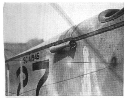
Fig. 55 .- Venturi tube on side of plane.
