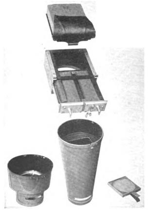
Fig. 44.—U. S. hand-operated aerial camera (type M) with 10 and 20 inch cones.
