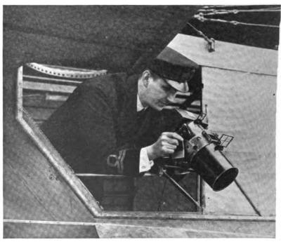
Fig. 185.—English"Type 18" hand camera on bracket for exposing through side window of flying boat.
