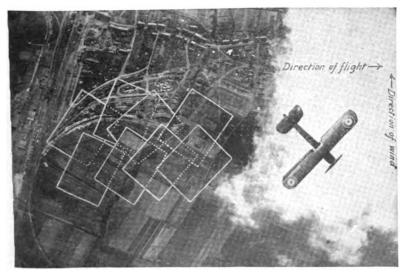
Fig. 188.—Unsatisfactory overlaps made when plane is "crabbing."
