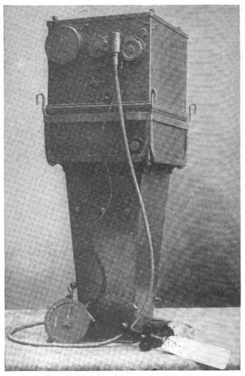
Fig. 54.—French model deRam automatic plate camera.
