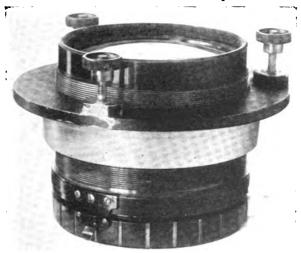
Fig. 18.—50 centimeter F/6 lens in U. S. standard mount, showing color filter retaining ring and catch. This ring screws down on the filter, and the catch is dropped into the nearest vertical groove to the tight position.
