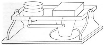
Fig. 80.—Diagram of camera linked to gyroscopic stabilizer.
