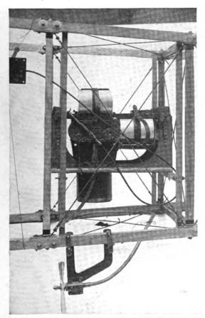
Fig. 83.—"L" camera and cradle mount in skeleton DeHaviland 4 fuselage, side view.
