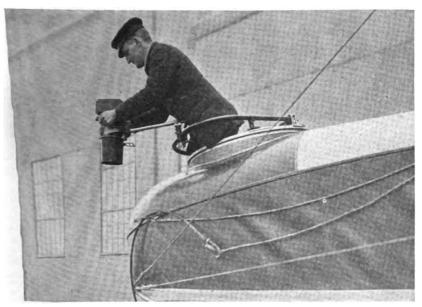
Fro. 186.—Camera mounted in bracket from forward cockpit of flying boat.
