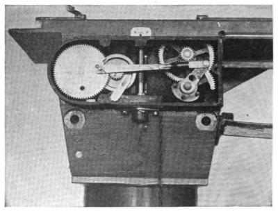
Fig. 51.—Mechanism of "L" camera.
