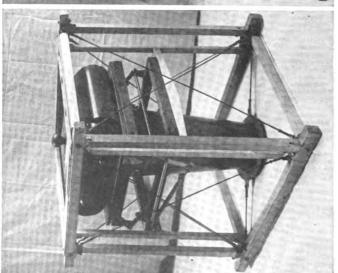
Fig. 97.—Section of fuselage of veneer construction affording superior accessibility to camera. F10. 96.—U. S. type "K" film camera on bell-crank mount, in camera bay of deHaviland 4. Vener frame at top of bay in place of usual cross-wices. made of the adequacy of the mounting, it must be said that the camera, as used, is perhaps the most eminently practical of all developed in the war, as its use on scouts testifies.
