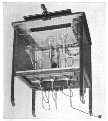
Fig. 119.-Interior of McIntire printer, showing lamps adjustable in position for "dodging."
