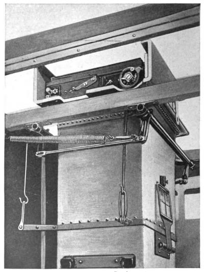
Fig. 86.—French spring and bell crank suspension.
