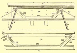
FIG. 15. — Machine for marbling paper. (Details of the brushing and graining device.)
