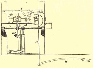
FIG. 27.—Fremy's machine. (Vertical section of the papercutting device.)
