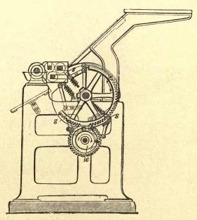
FIG. 5.-Steinmesse and Stollberg's gumming machine.
