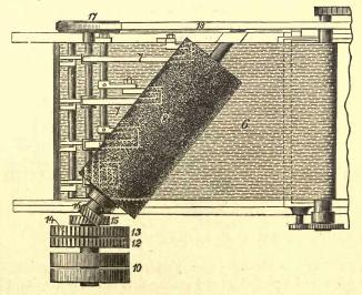
FIG. 7.-Machine for gumming paper.
