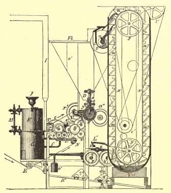
'FIG. 25.—Fremy's emery paper machine (longitudinal section).
