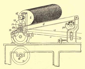
FIG. 6.-Machine for gumming paper.
