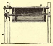
FIG. 28.—Fremy's machine. (Longitudinal section through the cutting cylinder in its frame.)
