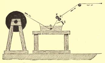
FIG. 3.-Apparatus for making wax paper.
