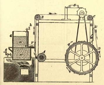
FIG. 9.-Apparatus for making endless hectograph paper.
