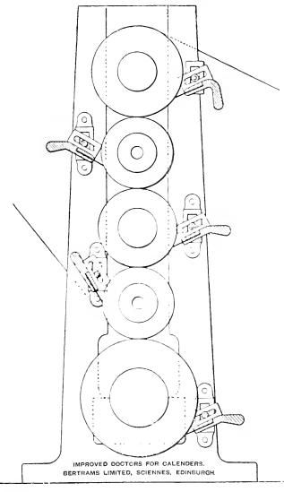
All the Continental mills have a doctor on each roll, effectually preventing the possibility of stamps, and sending the paper on to the reel perfectly clean, which is a saving of a large percentage of broke, besides facilitating the work in the finishing department. By the adoption of doctors, the danger to the fingers is considerably lessened, and the paper easier led through the calenders. I may also mention that I have seen, when making thick highly-machine-surfaced card-papers, such papers
