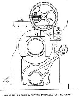
PRESS ROLLS WITH IMPROVED PARALLEL LIFTING GEAR.
