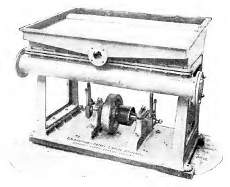
was constructed (as I am informed it has been since I commenced to write this article) with the same plate surface, but with less distance to travel, the impurities would be more quickly washed from the plate surface and on to the auxiliary strainer, thereby not giving the more minute particles time to pass through the plate.
