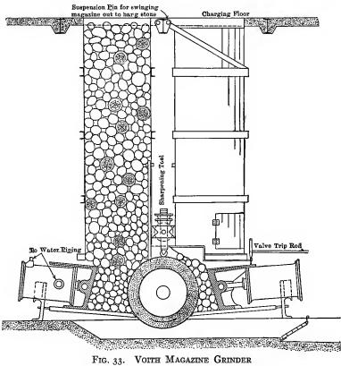
(2) Pressure employed in forcing the wood against the revolving stone.
