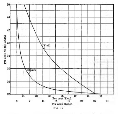
in that it was commercially unbleachable. Increasing the caustic to 28 per cent decreased the yield very greatly but produced easy bleaching fibre. When the caustic is brought up to 40 to 50 per cent of the weight of wood the form of curve suggests that its maximum cooking effect is nearly reached. This curve shows why 25 per cent of caustic soda is the most satisfactory for commercial work since if more is used the yield is too greatly reduced while if much less is employed the bleach required
