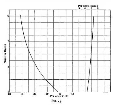
time for an increase from three to five hours causes a greater diminution in yield than an increase from seven to nine hours. Considering the questions of yield and bleach required the time factor is of much less importance than either the steam pressure or the amount of caustic added.
