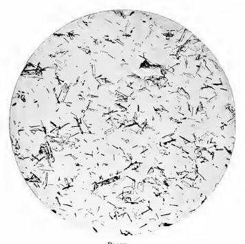
PLATE 29 Crown Filler. Magnification 100 diameters. Photographed by Bureau of Standards.
