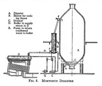
holding 14 to 15 cords of wood requires only one hour for the equivalent operations. The size of rotary digesters in American practice is generally about  $20 \times 7$  ft., while the vertical digesters range from 27 to 49 ft. tall by 7 to 10 ft. in diameter; one  $30 \times 8$  ft. will hold about 5.5 cords while one  $49 \times 10$  ft. will hold nearly 15 cords of wood.
