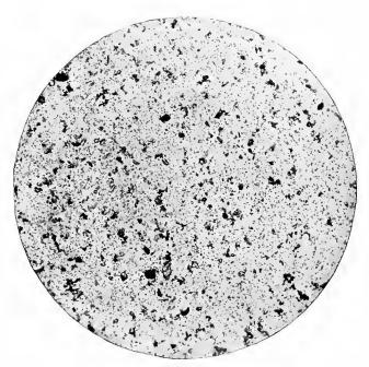
PLATE 28 English Coating Clay. Magnification 100 diameters. Photographed by Bureau of Standards.
