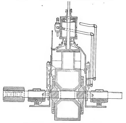
FIG. 32. THREE-POCKET GRINDER SECTIONAL ELEVATION
