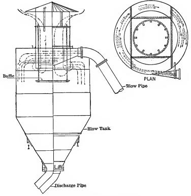
FIG. 16. BLOW TANK OR SEPARATOR
