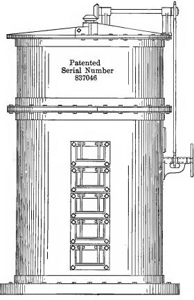
FIG. 23. VESUVIUS SULPHUR BURNER Courtesy of Valley Iron Works Company
