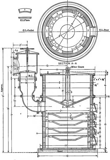
FIG. 24. VESUVIUS SULPHUR BURNER, SECTIONAL VIEW Courtesy of Valley Iron Works Company
