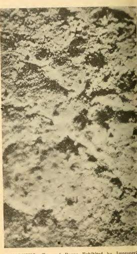
CHALKING.—Type of Decay Exhibited by Improperation Made Paint (magnified view).
