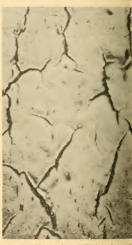
CRACKING.—Type of Decay Exhibited by Improperly Made Paint (magnified view).
