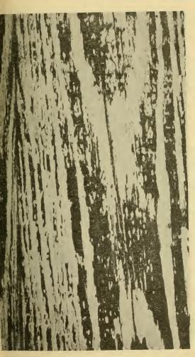
SCALING.—Type of Decay Exhibited by Improperly Made Paint (magnified view).
