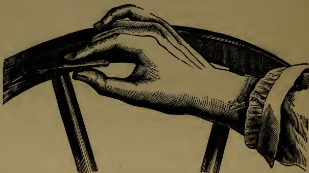
Fig. 11.—Showing the Position of the Hand in Striping the Rim of a Wheel.
