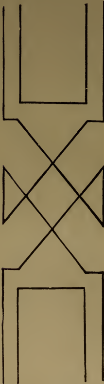
Fig. 18, Showing a "Break" in Striping.
