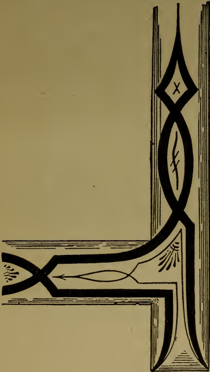
Fig. 17. Showing a method of Striping the Cross-bar and back end of the Shaft.
