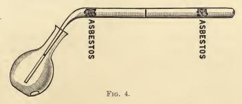
The mortar is then rinsed out with one washing of lime, and a plug of asbestos inserted in the tube, after which a further portion of lime is filled in. A layer of copper turnings, gauze
