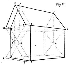
vanishing point will give the point 4 and the junction of 1 4, and 2 3 will give diagonals intersecting at o, whence a perpendicular is raised, meeting the line ff produced, at 5, then 1 5 and 2 5 supply the oblique lines of the projecting roof.
