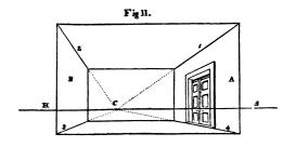
The lines 1 and 2, where the ceiling and walls meet, and 3 and 4, the lower limit of the walls, as well as the horizontal lines of the door and its panels, are, in that position of the spectator, all perpendicular to the plane of the drawing.
