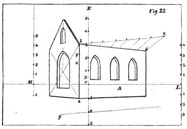
Determine the lower lines of the windows, as at n, on the line ab; and let no be the height of the chord of the arch from the bottom of the windows, and op the height from the chord to the apex of the arch, and from these points nop, draw lines towards the vanishing point of the line bd, which, by crossing the perpendiculars, will decide the heights of the windows. The point for the apex of each arch may be found by means of diagonals.
