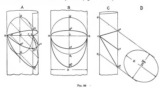
At C are sections of both cylinders taken parallel to the light, which falls at the angle  $\varphi$ . The top of the circle, at d, throws its shadow at  $d^*$ , the bottom  $d_1$  at  $d_1^*$ , and the center c at  $c^*$ .
