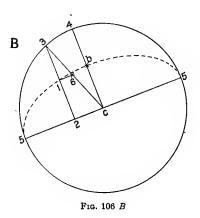
The symmetry of the ellipse affords, besides the given points 1 and 1, the six other points 1' and 1'' and 1'' and 1''' and 1'''. These eight points and the points 5 and 5, at the extremity of the Major Axis, being determined, the required ellipse can be drawn through them with sufficient precision.
