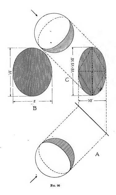
138. *Ellipsoids.*—The projection of a Prolate or Oblate Ellipsoid upon the Plane perpendicular to its axis is a circle; upon a plane parallel to the axis it is an ellipse similar to the generatrix of the Ellipsoid.
