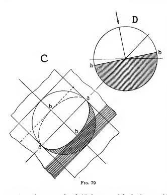
parallel to the projection of the light, will have its Line of Shade upon its outline and will again give the points aand a on the Line of Shade of the Sphere. The tangent cylinder, the projection of whose axis is at right angles with the projection of the rays of light, as appears in Cand D, will give two other points of the required Line of Shade, b and b.
