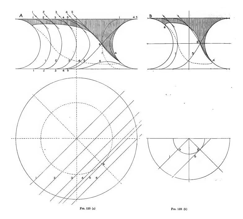
199. The Line of Shadow Upon the Scotia. Slicing.—Fig. 124 shows the elevation and plan of a Scotia cut by Vertical Planes set at 45° and parallel to the direction of the light, as in Fig. 123, with the Convex semi-circle of the upper edge of the Scotia casting its shadow upon the surface below, a surface which is convex in horizontal section and concave in vertical section.
