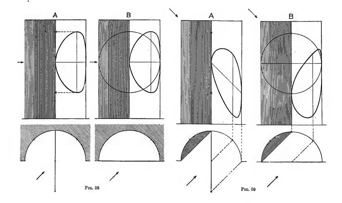
the shadows of the horizontal diameters are different, being a 45-degree right line in one case, as at A, and a 90-degree circular arc in the other, as at B, where the projection of this shadow coincides with the projection of one quadrant of the circle. The shadows of the two circles, though still symmetrical about the shadows of their diameters, differ accordingly, as appears in that figure.
