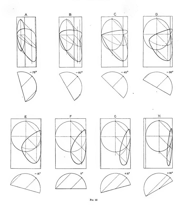
The shadow of the upper semicircle a d b falls at  $a d^* b$ , and that of the lower one  $a d_1 b$  at  $a d_1^* b$ . The line  $a c^* b$ , which is the shadow of the diameter a c b, is a true semiellipse, and the shadows of the semicircles which are symmetrical above and below this diameter, are also symmetrical above and below its shadow, and are also true semiellipses, as are also their projections.
