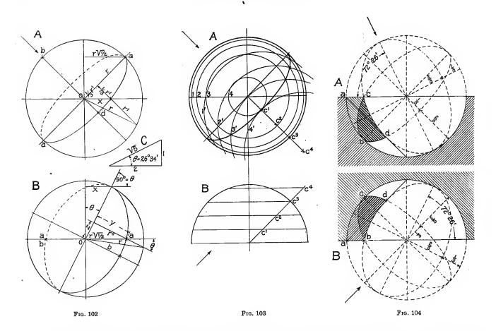
161. The Quarter Sphere.—The interior of the surface of the Quarter Sphere receives the shadow of part of the semicircle parallel to the plane of projection and of part of that perpendicular to it (Fig. 104). The line a b throws its shadow at b d, and the line a c at c d, the shadow of the point a falling at d.
