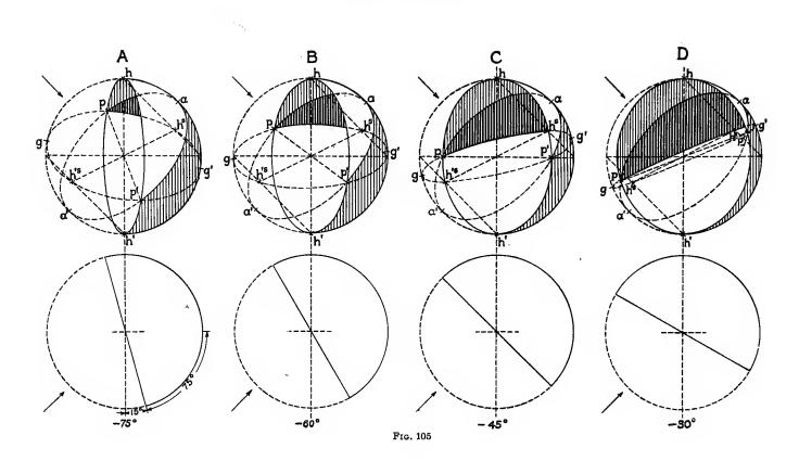
divided, and its projection is always the ellipse whose Major Axis is the diameter of the circle which makes 45 degrees with the horizontal diameter, and lies across the rays of light, and whose Minor Axes, lying parallel to those rays, measures, as in Fig. 78 A and B,  $\frac{2}{3}\sqrt[3]{3}-2\sqrt[3]{3}$ . This Major Axis is lettered a a'.
