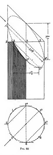
diameter of the ellipse which is parallel to the auxiliary Plane of Projection; and (4) of one of the 45-degree diameters of the vertical circle which cast the shadow.
