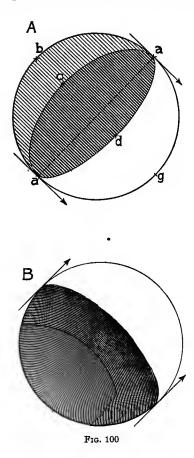
The Hollow Hemisphere, on the other hand, has upon its concave surface three lines, all of which are Great Semi-Circles, namely, (1) the Line of Shade upon the rim, which casts the shadow; (2) the Line of Shade and Shadow, which divides the shade from the shadow; and (3) the Line of Shadow, which divides the shadow from the light.
