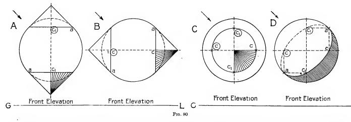
light three-quarters of the conical surface is in shade, two of which are out of sight; one of the elements that constitute the Line of Shade is on the outline of the cone that is nearest the light, and the other is on the near side of the cone, its projection coinciding with that of the axis, and half of the visible surface is in shade.
