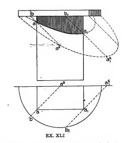
Thus the shadow of a horizontal circle falling upon a 45° plane is projected in a vertical circle, just as is the shadow of a horizontal line falling upon a vertical cylinder, as shown in Figs. 51 and 52.
