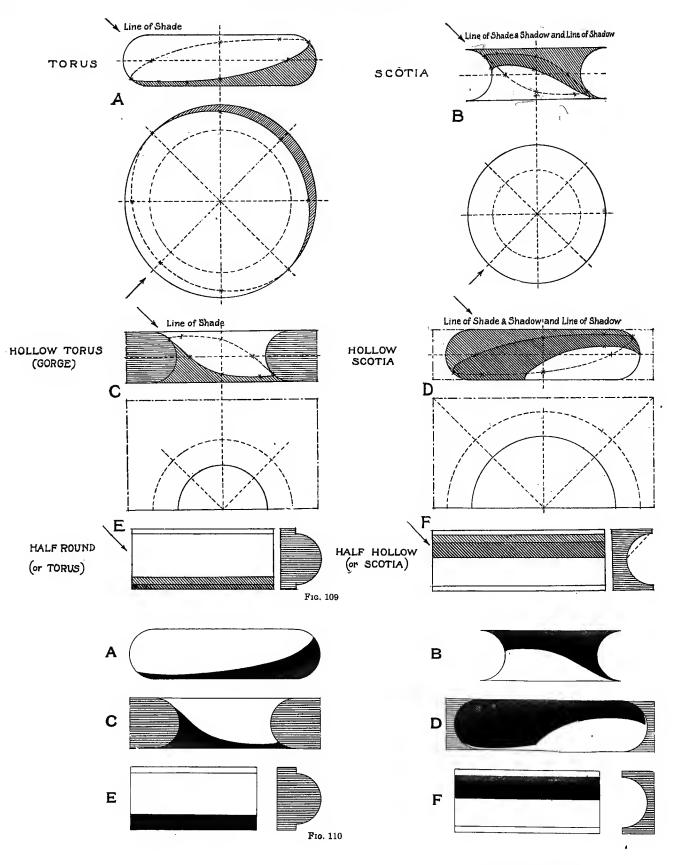
Scotia and the Hollow Scotia, being concave in section, cast shadows upon themselves (just as do the Hollow Cylinder, Hollow Cone, and Hollow Sphere). Like these they exhibit both shade and shadow, separated by the Line of Shade and Shadow.
