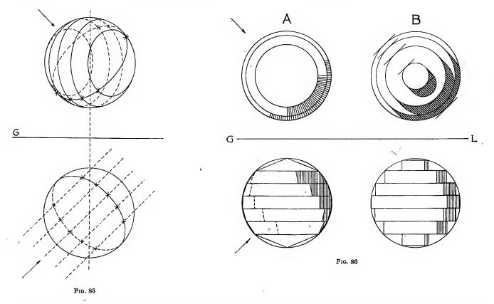
If the secant plane is, as in the figure, at 45 degrees with the vertical plane of projection, and perpendicular to the horizontal plane, these circles will be projected upon the horizontal plane in right lines at 45 degrees, as in the figure, and upon the vertical plane as Ellipses. But these are difficult to draw and the position of the tangent rays difficult to determine.
