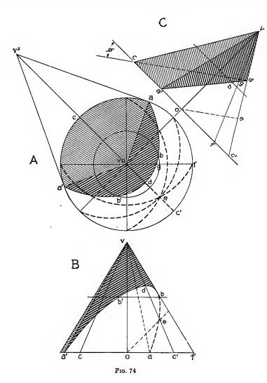
be a right line, as is shown at a'd, in Fig. 74 C. The Projection of this Elliptical Line of Shadow upon the horizontal plane, as shown in Fig. 74 B, is of course also an ellipse.
