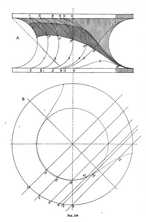
cast the shadows of these points upon the lower parts of these same curves, and lines drawn through them at 45° gives points of the required Line of Shadow at  $1^s$ ,  $2^s$ ,  $3^s$ ,  $4^s$ ,  $5^s$ , and  $6^s$ .
