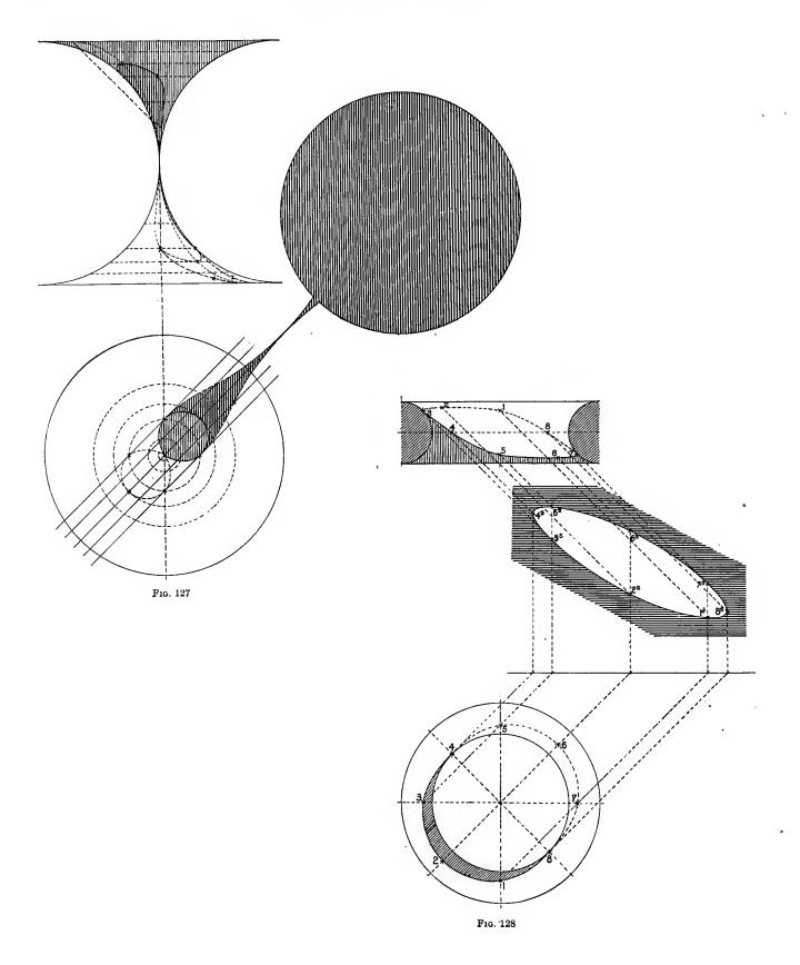
204. The Hollow Torus, or Gorge (Fig. 128).—The Line of Shade Upon the Gorge.—The Line of Shade of the Hollow Torus, or Gorge (Fig. 129), is, as has been said, the same as the Line of Shade and Shadow upon the Scotia (Fig. 122), the geometrical form of the two surfaces being identical.
