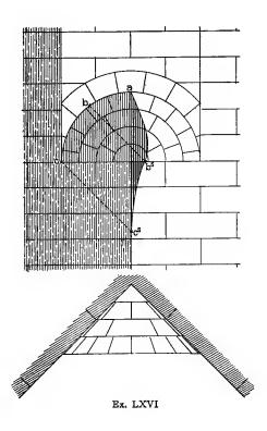
*Curved Pediments.*—Curved Pediments have generally an arc of 90 degrees. The Cymatium, or Gutter, rises at an angle of 45 degrees and projects in front just as much as along the eaves. The miter line at the intersection of the two lies in a vertical 45-degree plane.
