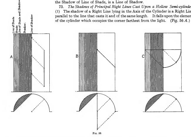
(2) The shadow of a diameter of the cylinder which is normal to the Plane of Projection is a quarter of an ellipse. Its projection is a Right Line, lying at 45 degrees, parallel to the projection of the rays of light, and extending from the Axis of the cylinder to the edge farthest from the light. (Fig. 56 B.) See Paragraph 65.
