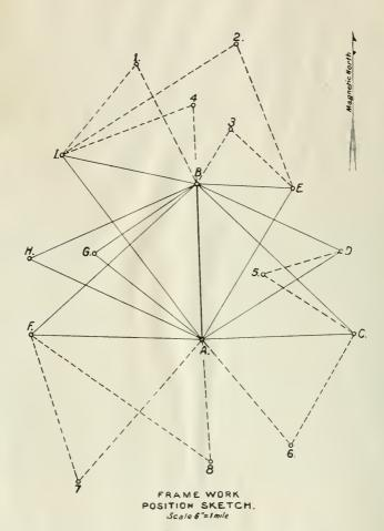
A. B. is the Base Line C.D.E.F. G.H.I. Points located by intersection 1.2.3.4.5.6.7.8 Points located by resection Intersection lines are plain & Resection lines are broken.
