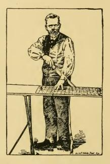
The cutter consists of a two edged cutting knife and a shear edged steel straight edge, fastened to the edge of the paste board. Marks' cutter is a first-class tool. Manufactured by James Marks, 666 Avenue D, Bayonne, N. J.
