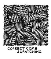
Over a well wetted down brick wall an ordinary sand-lime coat, mixed from 1 part lime and  $2\frac{1}{2}$  to 3 parts of sand is laid on to a thickness of about  $\frac{1}{4}$ . This coating is scratched with the comb and before it is left to set it is given a fine spray of water.
