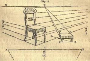
Figure 14 exhibits a parlour chair and a footstool. The student will observe that the chair stunds with the corner of its seat nearest to the spectator, the point of sight being in the middle of the picture. The receding sides of the chair have their respective parts regulated by diagonals to their vanishing points.
