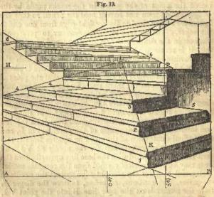
A flight of steps offers some peculiarities worthy of notice. In Fig. 19, the base AB regulates the angle of 60 degrees at 0, perpendicularly placed beneath the centre. The removal to the station is marked below the base line to S, and perpendicular to the point of sight P. The projected lines of the angle of 90 degrees at S are drawn right and left, till they intersect the horizontal line, and there determine the vanishing points V1 and V2.
