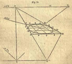
The base line AB must be drawn and divided into four equal parts, as 2, 4, 6; then from the base line, as in Fig. 10,
