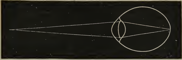
NEAR SIGHTED EYE SHOWING RAYS DIVERGING FROM A NEAR OBJECT SO THAT THEY COME TO A FOCUS ON THE RETINA.
