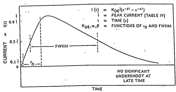
FIGURE 12. Double exponential waveform
