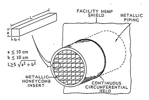
FIGURE 3. Typical waveguide-below-cutoff piping POE protective devices.
