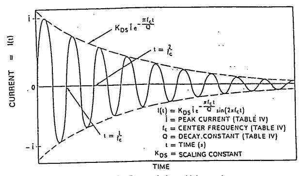
FIGURE 13. Damped sinusoidal waveform
