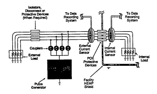
a. Common mode test configuration.
