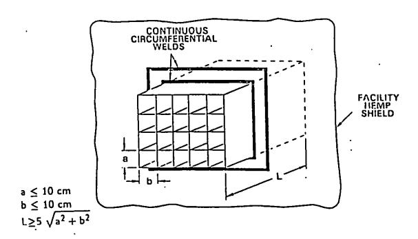
FIGURE 4. Typical waveguide-below-cutoff array ventilation POE protective device.
