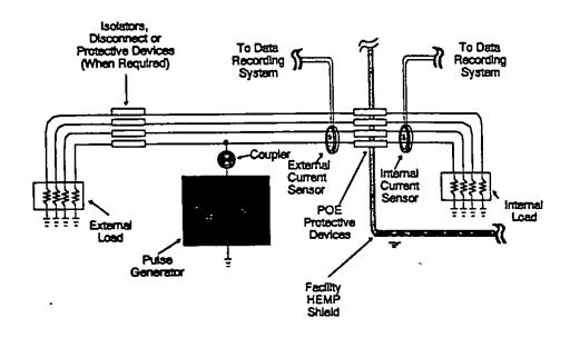
b. Wire-to-ground test configuration.
